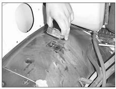
12. Loosen and remove the airbox mounting brack-
