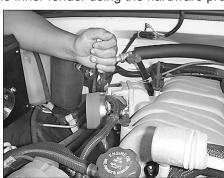
21.Install the silicone hose (08630) onto the throttle body and secure with a hose clamp provided.
