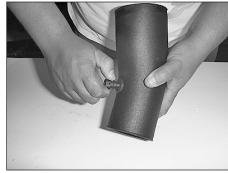
25. Install the air temperature sensor into the grommet
