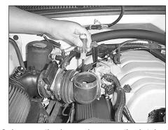
8. Loosen the hose clamp on the intake tube at the throttle body.
