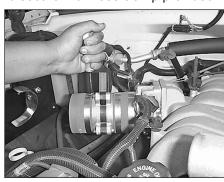
23. Attach the second silicone hose (08630) onto the flange of the mass air sensor and secure with hose clamp provided.
