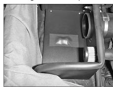
27. Apply the gasket provided onto heat shield to cover the exposed bolts.
