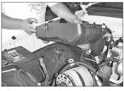
11. Release the air inlet duct from the inner fender. Lift firmly upward and remove the airbox base. NOTE: K&N Engineering, Inc., recommends that customers do not discard factory air intake.
