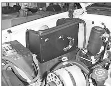
20. Install the heat shield assembly and secure to the inner fender using the hardware provided.
