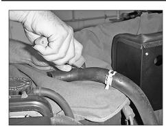
28. On models equipped with air injection, cut the air injection hose just past the first bend as shown.
