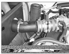
26. Install the K&N® intake tube into the silicone hose and tighten hose clamp.
