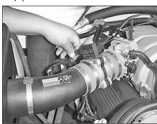
33. Reconnect the mass air sensor and air temperature sensor electrical connections.
