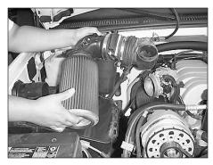
10. Remove the air intake assembly.
