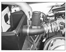
30. Secure the saddle bracket assembly to the intake tube with a hose clamp provided.
