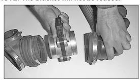
13. Remove the mass air sensor from the air intake assembly.
