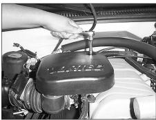
5. Loosen and remove the nut that retains the resonator.
