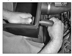
29. On models equipped with air injection, oil the A.I.R. filter with the oil provided. Insert the air filter through the small hole in the heat shield. Attach the air injection hose to the air filter and secure with the OE hose clamp.
