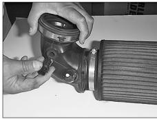
14. Remove the air temperature sensor from the air intake elbow.
