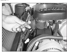
6. Loosen the hose clamp on the intake tube just beneath the resonator.
