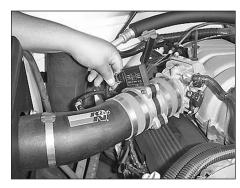
31. Tighten the saddle bracket hardware.
