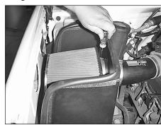
32. Install the air filter element and secure with hose clamp provided.
