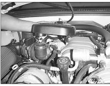
7. Remove the resonator as it will not be reused.
