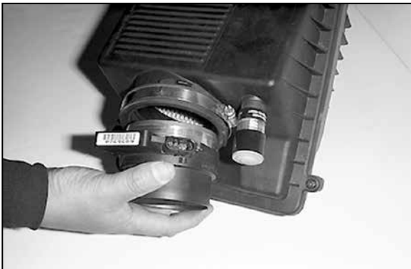
9. Loosen the hose clamp and remove the mass air sensor from the airbox.
