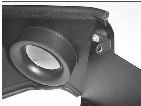
15. Attach the "L" bracket assembly to the heat shield. NOTE: Do not tighten completely at this time.
