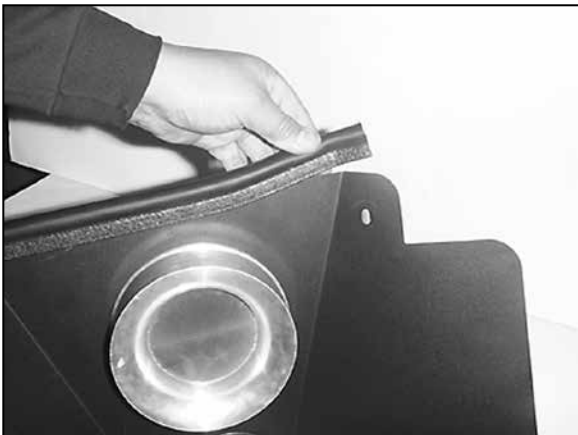
11. Install the trim seal onto the heat shield as shown. NOTE: Some cutting and trimming may be necessary to achieve best fit
