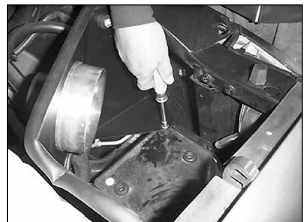
21. Secure the heat shield to the rubber mounted stud using the hardware provided.
