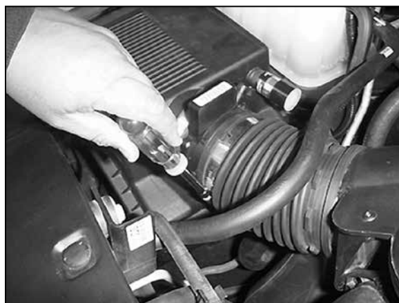
3. Loosen the hose clamp on the intake hose at the mass air sensor.
