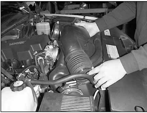
7. Detach the intake tube from the throttle body and remove the intake assembly.
