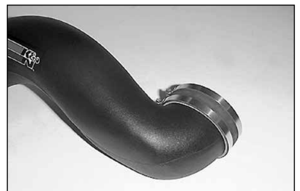
22. Install the 4"ID silicone hose onto the intake tube. NOTE: Do not tighten the hose clamps at this time.
