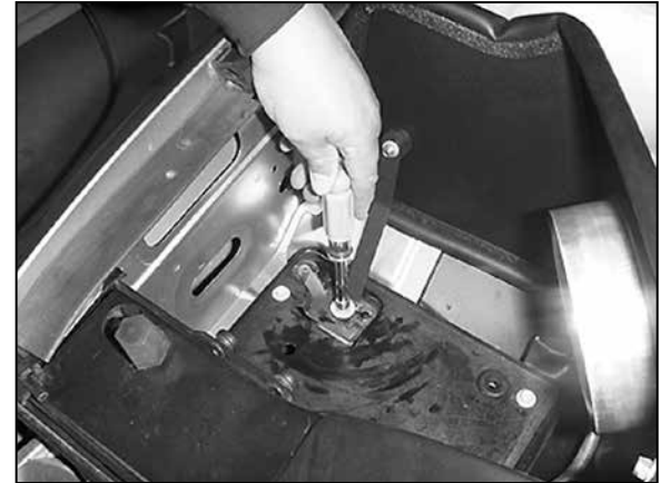
19. Secure the "C" bracket to the threaded hole in the airbox mounting tray using the bolt removed in step 16.
