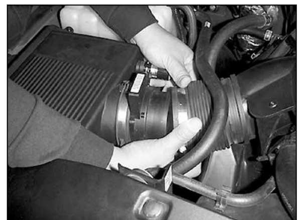
6. Detach the intake hose from the mass air sensor.
