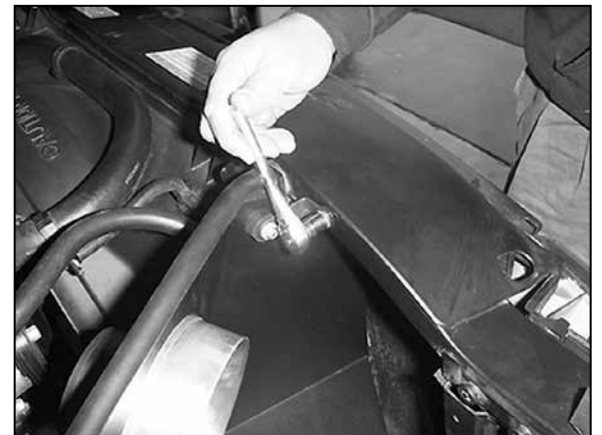
20. Secure the "L" bracket to the threaded hole in the radiator core support using the hardware provided.
