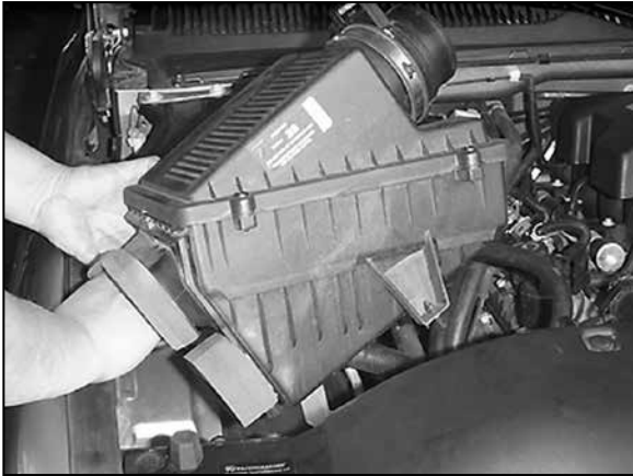
8. Pull firmly upward and remove the airbox. NOTE: K&N Engineering, Inc., recommends that customers do not discard factory air intake.
