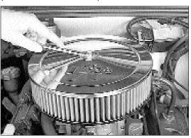
9. Install the provided washers and secure the Filtercharger assembly with the provided nylock nut.
