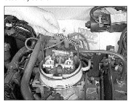
5) Loosen and remove the two factory air cleaner studs as shown.
