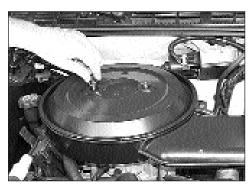
3. Loosen and remove the two wing nuts that secure the air cleaner assembly.
