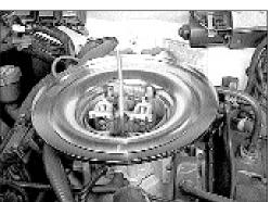
7. Install the K&N base plate on top of the factory plastic spacer as shown.
