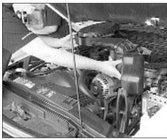
4) Remove the complete air cleaner assembly as shown.
