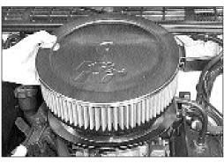
8. Install the K&N Filtercharger and the top plate onto the K&N base plate as shown.
