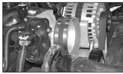
20. Install the provided silicone hose (08755) onto the throttle body with provided hose clamps.
