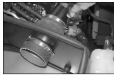
21. Install the intake tube onto the vehicle; then align the tube with the mass air sensor and then tighten hose clamp.
