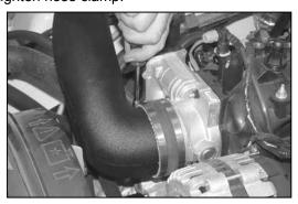
22. Align the intake tube with the throttle body then tighten the hose clamps.
