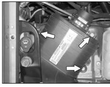
7. Remove the 3 10mm bolts that retain the air box onto the vehicle.
