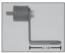
13. Install the 1" long rubber mounted stud onto bracket as shown.
