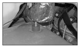
14. Install the rubber mounted stud onto the vehicle as shown.
