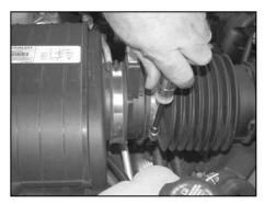
5. Loosen the hose clamp at the mass air sensor.
