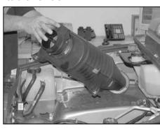
8. Remove the air box from vehicle as shown. NOTE: K&N Engineering, Inc., recommends that customers do not discard factory air intake.
