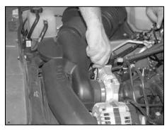
4. Loosen the hose clamp at the throttle body.
