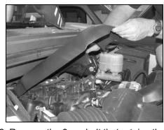
2. Remove the 8mm bolt that retains then engine cover onto the engine then remove the cover from vehicle.
