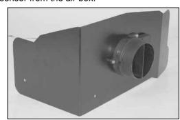
10. Install the mass air sensor onto the heat shield with the provided hardware.
