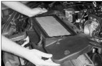
6. Loosen and remove the four bolts that retain the air box base to the radiator core support, then remove the lower air box assembly.
