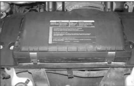
4. Release the two clips that retain the air box top to the air box base.
