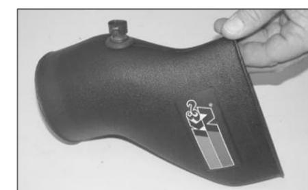
13. Install the temp sensor into the K&N intake tube as shown.
