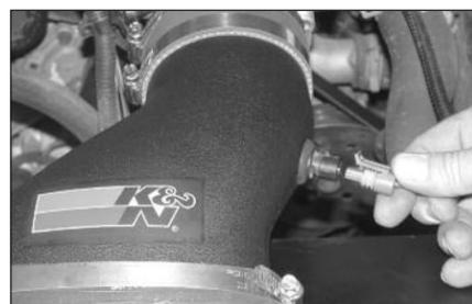
19. Reconnect the air temp sensor electrical connection.
