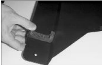
8. Install the rubber cushion onto the heat shield as shown.
