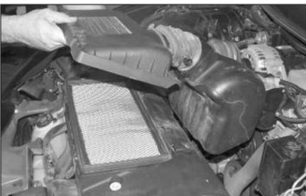
5. Remove intake from throttle body, then remove the entire upper air intake assembly.
