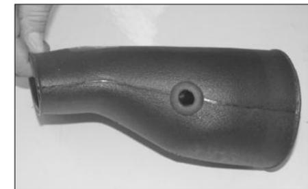
11. Install the grommet into the K&N intake tube as shown.
