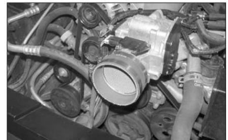
10. Install the provided silicone hose (08621) onto the throttle body with the provided hose clamps.
