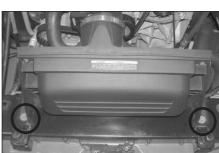
7. Remove the two bolts, which secure the air box to the core support.
