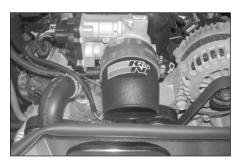
15. Install the K&N intake tube into the silicone hose at the throttle body and secure with the provided hose clamp.
