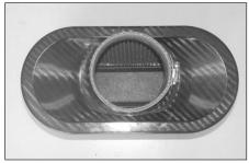
22. Note the flange of the air filter is offset. The offset is to the top of the filter.
