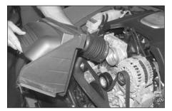
8. Loosen the hose clamp that secures the stock intake tube to the throttle body, and then remove the complete intake assembly from the vehicle.
