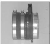
16. Install the provided silicone hose (08615) onto the engine side of the mass air sensor and secure with the provided hose clamp.
