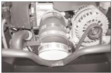
17.Install the mass air sensor assembly onto the K&N intake tube and secure with the provided hose clamp.
