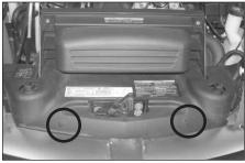
4. Release the center locking pins in the twocore support cover holding clips, and then pull the holding clips out.
