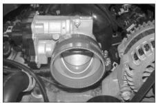
14. Install the provided silicone hose (08625) onto the throttle body and secure with the provided hose clamp as shown.
