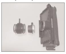
9. Loosen the two hose clamps securing the mass air sensor to the stock air box and intake tube, and then remove the mass air sensor.
