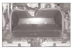
13. Install the heat shield assembly onto the air box mounting points and secure with the factory air box mounting bolts.
