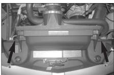
5. Remove the two 10mm nuts, which hold the core support cover onto the air box.
