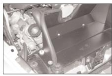
18. Install the two provided nylon spacers onto each side of the air box mounting studs as shown.
