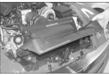
6. Lift the core support cover up and remove it from the vehicle.
