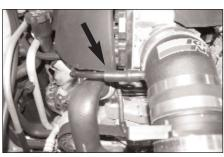
20. Install the provided crank case vent hose onto the K&N intake tube and then connect the factory vent tube into the K&N vent hose as shown.
