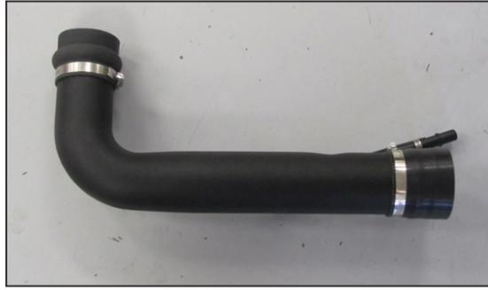
12. Install the provided hump coupler (08185) onto the K&N® intake tube as shown and secure with the provided hose clamp.
