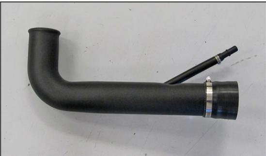
11. Install the provided step coupler (08429) onto the K&N® intake tube.
