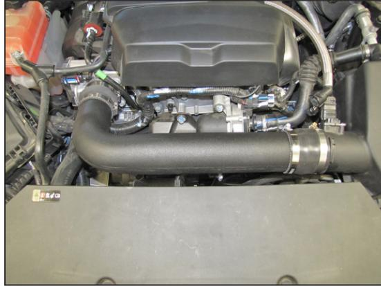
13. Install the K&N® intake tube assembly onto the air box and then onto the throttle body. Adjust the tube and coupler for best fit and then secure with the provided hose clamps.
