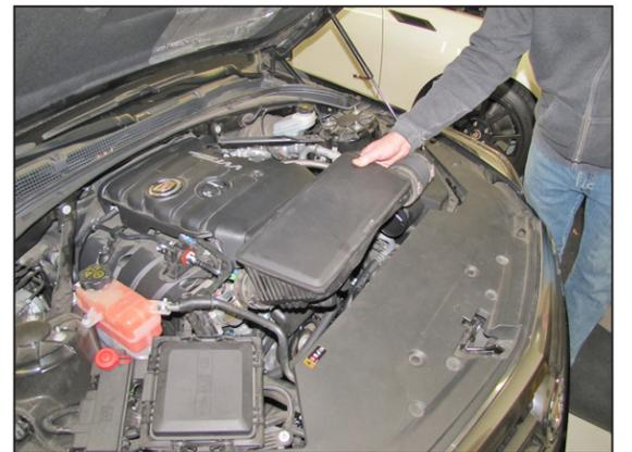
5. Remove the intake plenum from the throttle body and then from the air filter housing.
