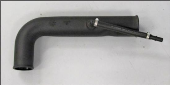
10. Install the crank case vent assembly onto the fitting installed into the K&N® intake tube and secure with the provided hose clamp.
