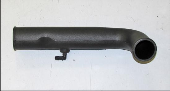
8. Install the provided vent fitting into the K&N® intake tube as shown.
