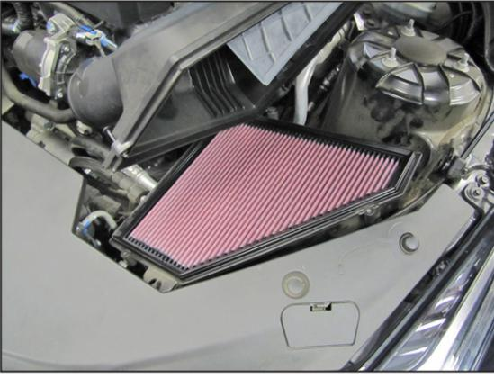
7. Install the K&N® air filter and then secure the lid with the factory hardware.
