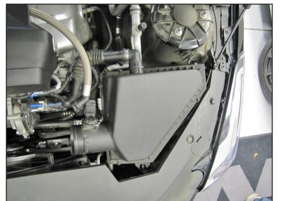
6. Loosen the four screws securing the air box lid and then remove the factory air filter.
