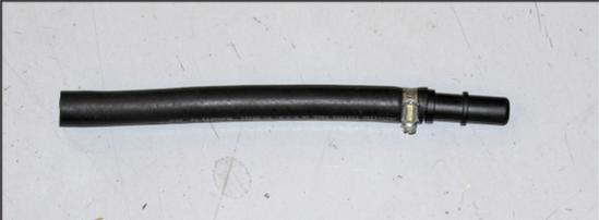
9. Install the provided quick disconnect union into the provided vent hose and secure with the hose clamp provided.
