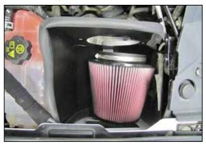
10. Set the  $K\&N^{\otimes}$  air filter into the heat shield as shown.
