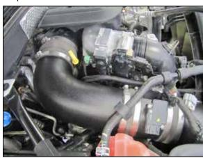
18. Install the K&N® intake tube into the hose at the Mass air sensor and then into the hose at the turbo inlet, adjust the tubes for best fit and then secure with the provided hose clamps.
