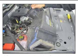
6. Lift up and remove the air box from the vehicle. NOTE: K&N Engineering, Inc., recommends that customers do not discard factory air intake.
