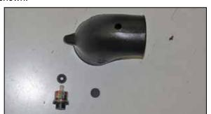
11. On vehicles equipped with a filter minder, remove the filter minder and grommet from the intake tube and install into the K&N intake tube as shown. On vehicles that are not equipped with a filter minder, drill the hole in the K&N intake tube out to 7/8"ID and then install the provded plug into the tube.
