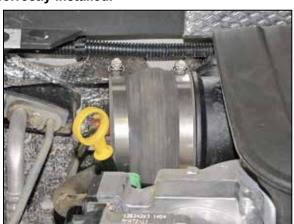
17. Install the provided hump hose (08633) onto the turbo inlet and secure with the provided hose clamp.
