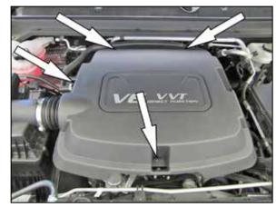
6. Loosen the two bolts that secure the rear of the intake plenum and remove the two forward bolts that secure the plenum.
