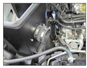
16. Install the provided hump coupler (06899) onto the filter adapter and secure with the provided hose clamp.
