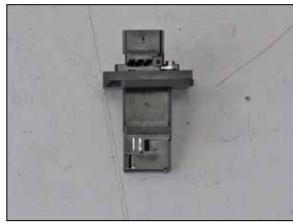
20. Install the factory mass air sensor into the K&N® adapter assemble and secure with the provided hardware.
