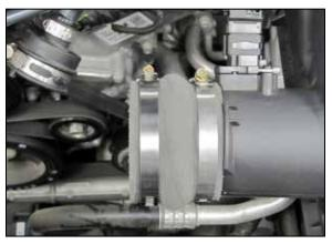
12. Install the provided hump coupler hose (08171) onto the Mass air sensor outlet and secure with the provided hose clamp.
