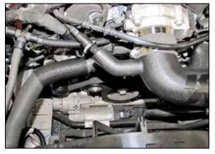
15. Connect the factory EVAP hose quick connector to the quick connector installed into the K&N<sup>®</sup> intake tube.
