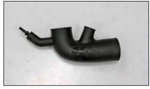
13. Install the provided quick disconnect NPT fitting into the K&N<sup>®</sup> intake tube as shown. NOTE: Plastic NPT fittings are easy to cross thread. Install the vent fitting "hand" tight, then turn it two complete turns with a wrench.
