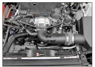
14. Install the K&N<sup>®</sup> intake tube into the coupling hose at the air box and then into the coupler at the throttle body, adjust the tube for best fit and then secure with the provided hose clamps.
