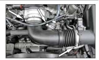
5. Loosen the three hose clamps that secure the
