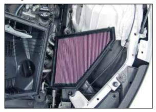
10. Remove the upper air filter housing and replace the factory air filter with the provided K&N® air filter. Reinstall the factory air filter housing and secure with the factory screws.
