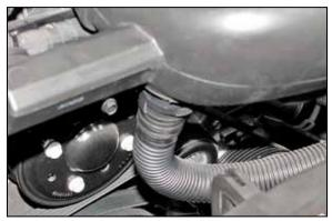
4. On vehicles equipped with an engine sound tube, release the sound tube quick disconnect fitting and disconnect the sound tube from the factory intake tube. intake tube and crank case vent tube and remove the intake tube from the vehicle.
