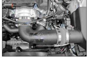
16. Connect the crank case fitting onto the K&N® intake tube and secure with the provided hose clamp.
