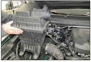
5. Remove the complete air filter housing from the
