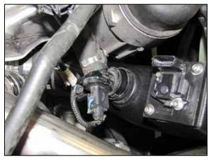
24. Connect the vent Quick disconnect fitting onto the fitting installed into the K&N® intake tube.
