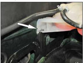
15. Remove the nut shown that secures the coolant reservoir.
