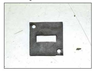
18. Install the provided gasket onto the  $K\&N^{\mbox{\scriptsize @}}$  mass air sensor adapter.
