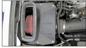
17. Install the K&N® air filter housing lid onto the filter housing and secure with the provided hardware.
