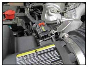
2. Slide the red locking tab back and then release the mass air sensor electrical connection.
