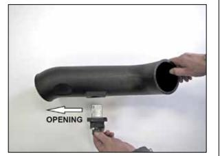
11. Install the sensor assembly into the K&N® intake tube and secure with the provided hardware. NOTE: Be sure to install the sensor in the correct direction, the opening in the sensor should be pointed towards the filter end of the tube.
