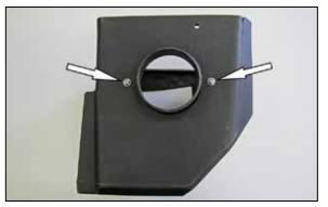
6. Install the filter adapter into the K&N<sup>®</sup> air filter housing and secure with the provided hardware.
