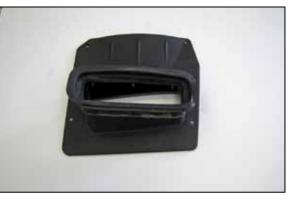
16. Install the bellows onto the K&N® air filter housing lid and secure with the factory retaining clips.
