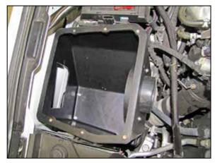
7. Install the K&N<sup>®</sup> air filter housing into the vehicle and secure it to the factory housing mounting plate fastener location with the hardware removed in step 5.
