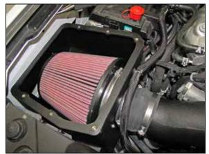
14. Install the K&N® air filter into the air filter housing and then onto the filter adapter. Secure the filter with the provided hose clamp. NOTE: Be careful installing the filter into the housing to avoid catching the side edges of the housing and damaging the filter. NOTE: Drycharger<sup>®</sup> air filter wrap; part # RC-5139DK is available to purchase separately. To learn more about Drycharger® filter wraps or look up color availability please visit http://www.knfilters.com®.
