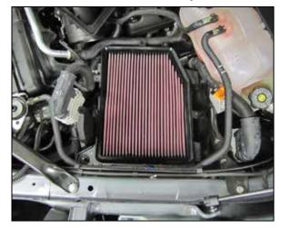
4. Loosen the three bolts that secure the upper air filter housing and then lift off the housing and replace the factory air filter with the K&N<sup>®</sup> air filter. Reinstall the upper housing and secure with the factory bolts.
