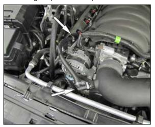
9. Install the crank case vent assembly onto the valve cover port and the fitting installed into the  $K\&N^{\mbox{\tiny $\$$}}$  intake tube as shown.
