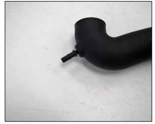
5. Install the provided quick disconnect fitting into the  $K\&N^{\otimes}$  intake tube as shown.
