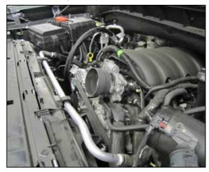
6. Install the appropriate coupler onto the throttle body and secure with the provided hose clamp.5.3L engines will use coupler #08497, 6.2L engines will use coupler #084107.
