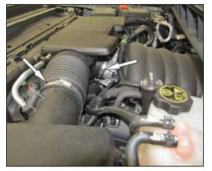
3. Loosen the hose clamps that secure the intake plenum to the air filter housing and the throttle body. Rotate the plenum up counter clockwise to disengage it from the mount and then remove the plenum from the vehicle.
