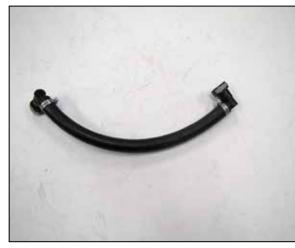
8. Assemble the crank case vent assembly as shown using the provided components.
