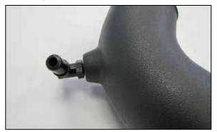
8. Install the provided  $90^{\rm o}$  vent fitting into the K&N  $^{\rm o}$  intake tube as shown.
