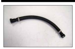
10. Assemble the crank case vent hose assembly as shown.
