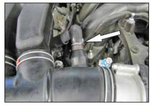
3. Release the spring clamp and then disconnect the crank case vent hose from the factory intake tube.
