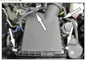
6. Release the three air filter housing clips and then lift off the upper air filter housing and remove the intake tube assembly from the vehicle.
