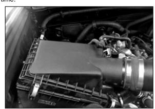
11. Reinstall the factory air filter housing and secure with the factory retaining clips.
