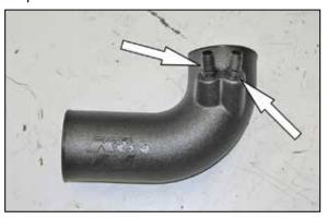
9. Install the provided vent fittings into the K&N® intake tube as shown.
