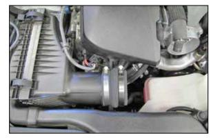
7. Install the coupling hose (08699) onto the air filter housing and secure with the provided hose
