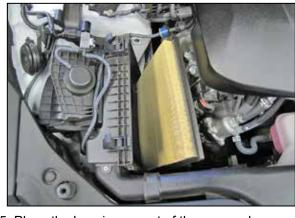
5. Place the housing up out of the way and remove the stock air filter from the lower housing.
