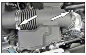
4. Loosen the hose clamps securing the factory intake tube to the throttle body and air filter housing and then remove the factory intake tube from the vehicle.
