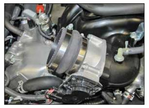
7. Install the provided hump coupler (08699) onto the throttle body and secure with the provide hose clamp.
