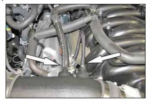
11. Connect the union into the factory crank case vent hose and then connect the open end onto the fitting installed into the  $K\&N^{\mbox{\tiny $\$$}}$  intake tube. Then connect the fuel pressure regulator vent hose to the fitting installed in the  $K\&N^{\mbox{\tiny $\$$}}$  intake tube.
