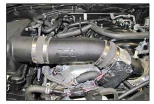
9. Lift up the upper air filter housing, install the K&N<sup>®</sup> intake tube into the coupling hoses and then reinstall the air filter housing. Secure the air filter housing with the factory clips, adjust the intake tube for best fit and then secure with the provided hose clamps.
