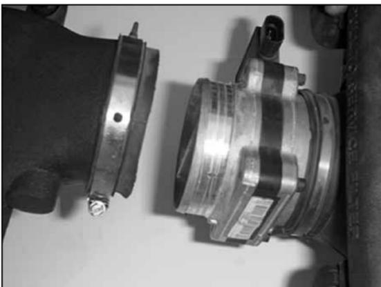
9. Loosen the hose clamp and detach the stock intake tube from the mass air sensor.
