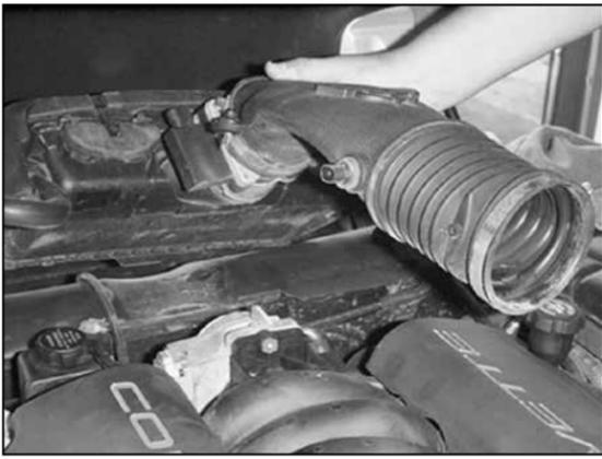
7. Detach the intake hose from the throttle body and remove the entire air intake assembly.
