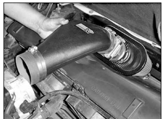
23. Install the K&N® intake assembly.
