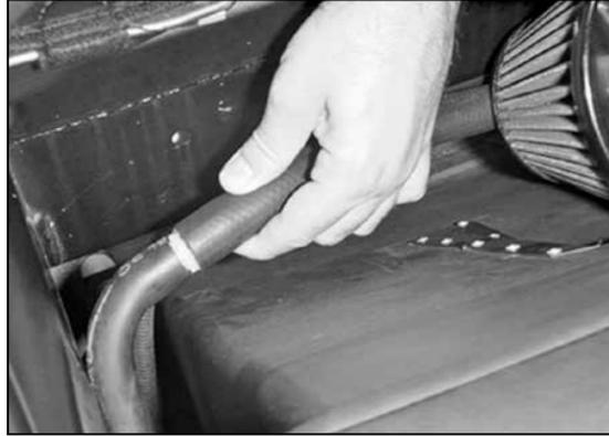
49. Attach the air injection hose to the hose mender.
