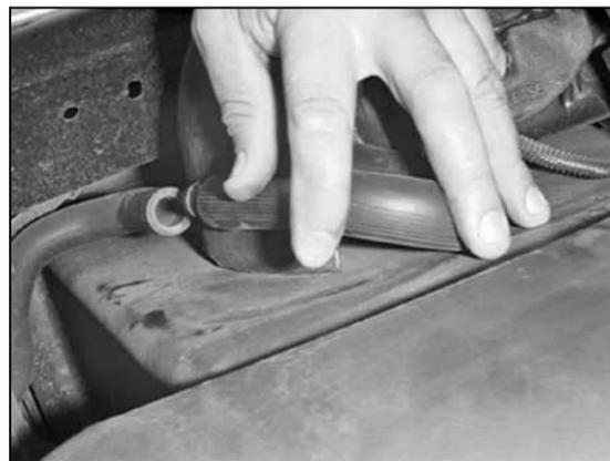
3. Disconnect the air injection vent hose.
