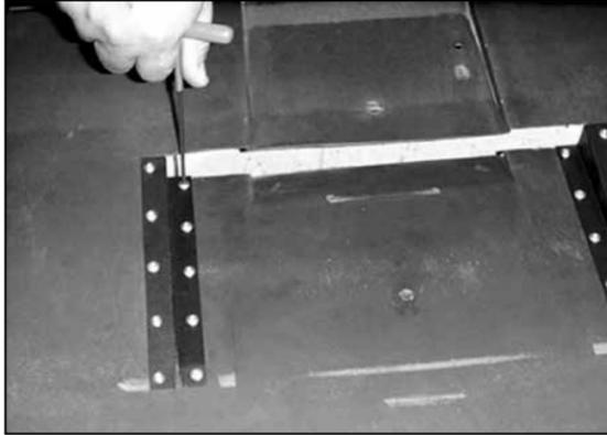
42. Secure the flap to the brackets with the hardware provided.
