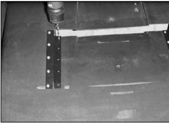
41. Drill out the five inner holes of each bracket.
