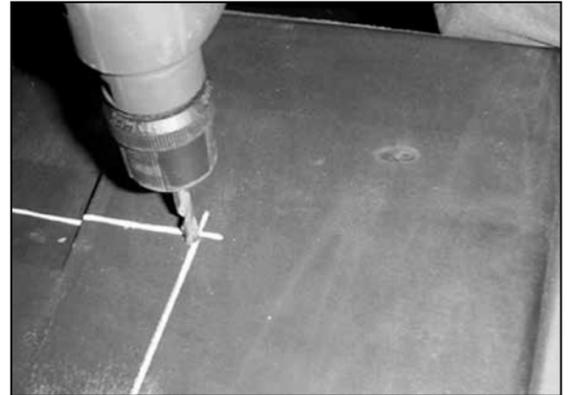
36. Using a 5/16" drill bit, drill a hole where the horizontal and vertical lines intersect.
