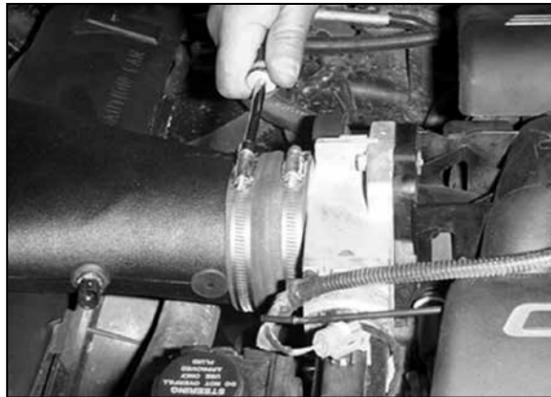
50. Attach the silicone hose to the throttle body and tighten the hose clamps.
