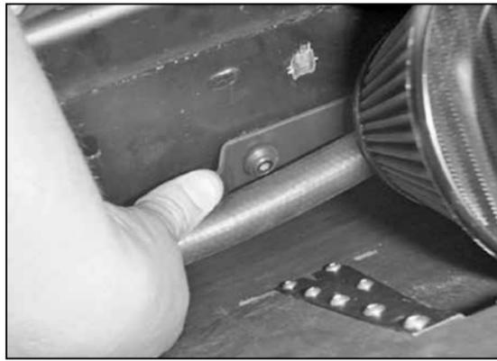
48. Install the angled bracket onto the original airbox mounting points.
