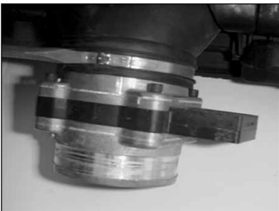
10. Remove the mass air sensor hose clamp.
