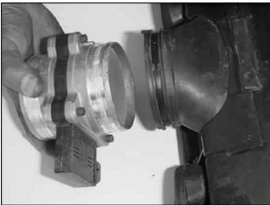
11. Remove the mass air sensor from the airbox.
