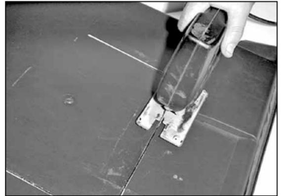
37. Using a jigsaw, cut along the horizontal and vertical lines.
