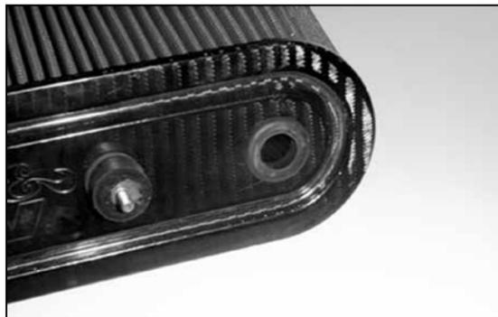
15. Install the 5/8" ID grommet and the rubber mounted stud into the top plate of the Air filter element.
