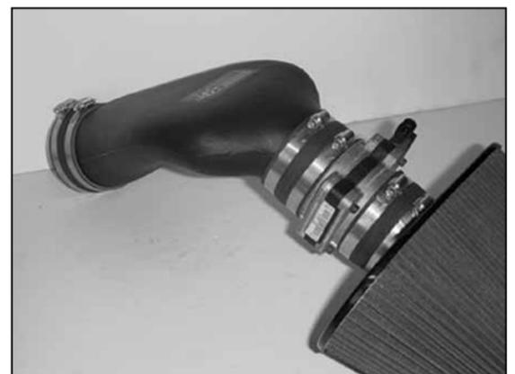
22. Assemble the intake tube and Air filter element assemblies.
