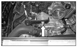
7a. On vehicles equipped with an intake resonator, remove the nut shown that secures the resonator bracket; remove the resonator bracket from the engine.
