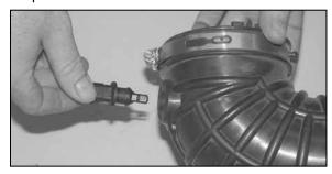
15. Remove the air temperature sensor from the factory intake tube.
