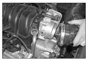
4. Loosen the hose clamp that secures the intake tube to the throttle body and pull the intake tube off of the throttle body.
