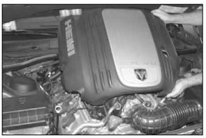
2. Lift up on the engine cover to loosen it from the mounts, and then remove the cover from the vehicle.
