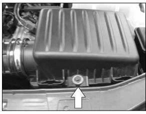
6. Loosen and remove the airbox mounting bolt as shown.
