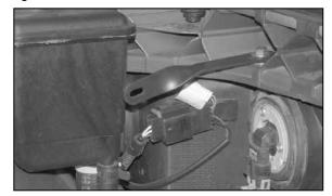
8. Install the twist bracket (070772) onto the core support using the hardware provided through the existing hole as shown.
