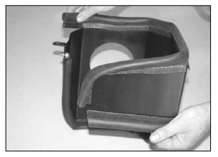
10. Install the two pieces of edge trim onto the heat shield as shown, be sure to leave a gap at the bracket mounting locations.
