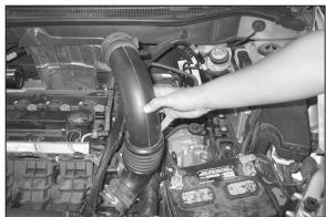
10. Remove the stock intake tube from the vehicle. NOTE: Be sure to unclip the wiring harness from the intake tube as you remove the tube from the vehicle.
