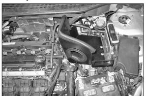
25. Install heat shield onto the mounting studs and secure with the two nuts removed in step #12 and the provided hardware.
