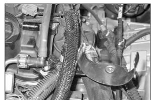
21. Install the tube mounting bracket assembly onto the valve cover stud and secure with the provided hardware.
