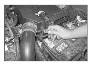
5. Depress the locking tab and disconnect the inlet air temperature sensor's electrical connection.
