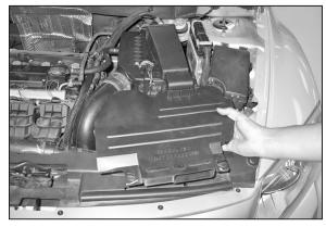
4. Remove the fresh air duct from the stock air filter housing and radiator core support.
