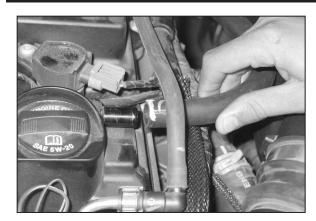
7. Disconnect the crank case vent hose from valve cover.
