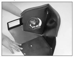
24. Install the short edge trim into the tube pass through hole as shown.
