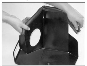
23. Install the long edge trim along the top of the heat shield as shown.
