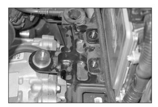
22. Install rubber mounted stud using the large fender washers provided.
