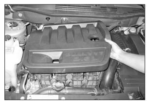
2. Pull up firmly to dislodge the engine cover from the mounting grommets. Then remove the engine cover from the vehicle.
