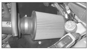
29. Install the K&N® air filter and secure with the provided hose clamp.
