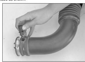
15. Remove the air temperature sensor from the factory intake tube as shown.
