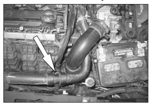
9. Loosen the hose clamp at the lower end of the stock intake tube from the vehicle.
