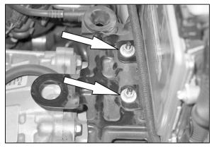
12. Remove the two air box mounting nuts shown. **NOTE: These nuts will be reused in a later step**.
