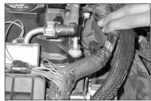
20. Place one washer onto the valve cover stud as shown.
