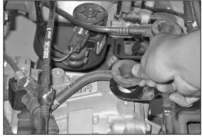
11. Remove the air box mounting grommet shown.
