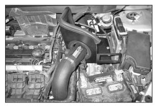
26. Install the K&N® intake tube into the silicone hose and align onto the saddle clamp. Then secure with the provided hose clamps. Tighten bolts in #21.
