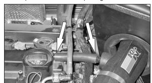
27. Install the provided crank case vent hose onto the valve cover. Then onto the fitting installed into the K&N® intake tube.
