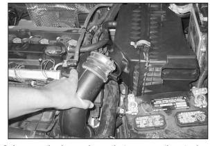
6. Loosen the hose clamp that secures the stock intake tube to the factory air filter housing.
