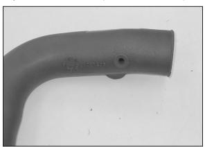
14. Install the supplied grommet into the intake tube as shown.
