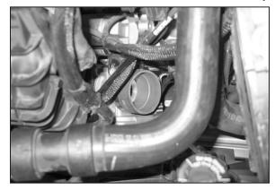
13. Install the silicone hose (08108) onto throttle body and secure with the provided hose clamp.
