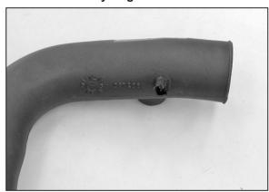
16. Install the air temperature sensor into the grommet.
