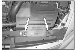
3. Rotate the fresh air tube fasteners counter clockwise to unlock them from the radiator core support.
