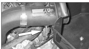
28. Reconnect the air temperature sensor electrical connection.
