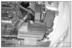
30. Install the fresh air duct into the heat shield and onto the core support. Then secure with the factory quarter turn fasteners.
