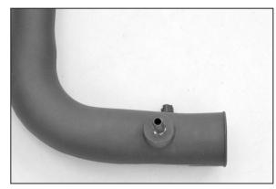
17. Install the supplied 1/4" npt vent fitting into the threaded boss in the K&N® intake tube as shown. NOTE: Plastic NPT fittings are easy to cross thread. Install the vent fitting "hand" tight, then turn it two complete turns with a wrench.
