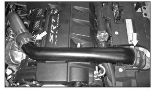
6. Loosen the two hose clamps that secure the intercooler transition tube. Then remove the intercooler transition tube.
