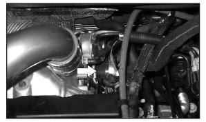
15. Install the provided silicone hose (08095) onto the turbo inlet and secure it with the provided hose clamp. 20. Install the provided crank case vent hose to the 1/4NPT X 1/2" on the K&N<sup>®</sup> intake tube and then attach the other end to the vent port on the valve cover as shown.
