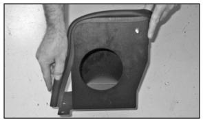
22. Install the provided edge trim onto the heat shield as shown.
