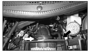
9. Loosen the hose clamp that secures the factory intake hose to the air box. Then unhook both the intake hose and vent hose from the air box.
