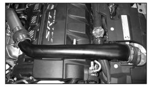
27. Reinstall the intercooler tube and secure with the factory hose clamps.
