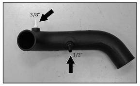
18. Install the two 1/4NPT fittings into the K&N<sup>®</sup> intake tube as shown.
