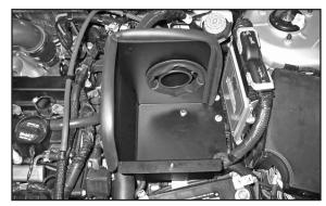
24. Install the heat shield onto the rubber mounted stud installed during step #13 and onto the ECU mounting studs. Then secure the heat shield with the factory ECU mounting bolts and hardware provided.
