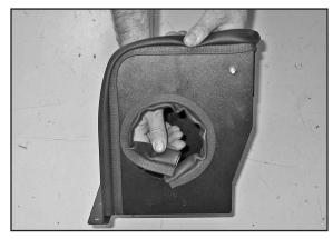
23. Install the provided edge trim into the hole of the heat shield as shown.
