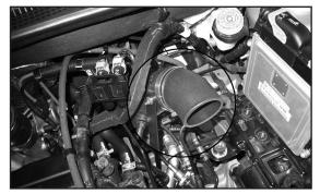
19. Install the K&N<sup>®</sup> intake tube into the silicone hose at the turbo inlet and align with the mounting bracket, then secure with the provided hose clamps.
