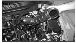
11. Loosen the hose clamp that secures the intake hose to the turbo inlet and then remove the intake tube from the vehicle.
