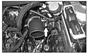
21. Attach the remaining vent hose to the 1/4NPT X 3/8" vent fitting installed in the K&N<sup>®</sup> intake tube.
