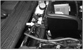
25. Secure the vacuum solenoids to the stud on the back of the heat shield using the provided hardware.
