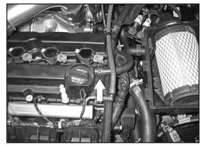
2. Unlock the two fresh air retaining clips by turning a  $\frac{1}{4}$  turn counter clockwise.
