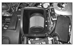
28. Install the K&N<sup>®</sup> air filter onto the intake tube and secure with the provided hose clamp. NOTE: Drycharger<sup>®</sup> air filter wrap; part # RX-4990DK is available to purchase separately. To learn more about Drycharger<sup>®</sup> filter wraps or look up color availability please visit http://www.knfilters.com<sup>®</sup>.
