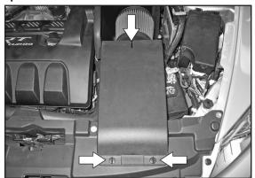
29. Install the fresh air intake duct onto the core support and heat shield, and then secure with the factory  $\frac{1}{4}$  turn clips and hardware provided.
