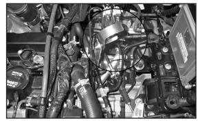
17. Secure the intake tube mounting bracket to the driver's side of the tab on the transmission using the provided hardware.
