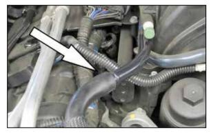
7. Disconnect the crank case vent hose from the crank case vent tube.
