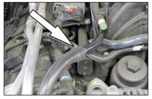
32. Connect the open end of the crank case vent hose to the factory crank case vent tube as shown.
