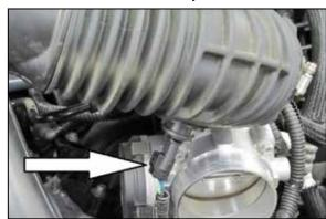
6. Lift up the intake tube, disconnect the inlet air temperature electrical connection then remove the intake tube from the vehicle.
