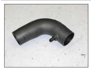
30. Install the provided NPT crank case vent fitting into the  $K\&N^{@}$  intake tube as shown.
