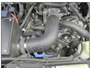
34. Install the K&N® intake tube into the hump coupler and then into the throttle body coupler, adjust the tube for best fit and then secure with the provided hose clamps. Reconnect the inlet air temperature sensor electrical connection.
