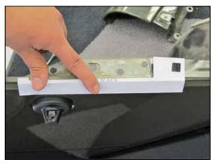
46. Using the provided template, mark the fender where the excess material needs to be removed from the fender.
