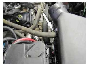
**4.** Disconnect the crank case vent hose from the upper air filter housing.
