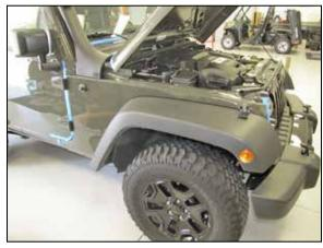
49. With an assistant, temporarily reinstall the fender onto the vehicle but do not secure it at this time. Adjust the snorkel for best fit and then secure the snorkel bracket to the inner cowl and the outer cowl to the snorkel with the factory hardware.
