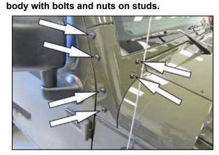
7. Using a T40 socket, remove the six bolts that secure the corner cap and then remove the corner cap
