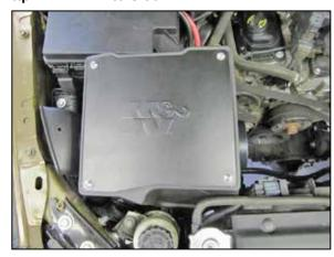
27. Install the air filter housing lid and gasket and secure with the provided hardware.
