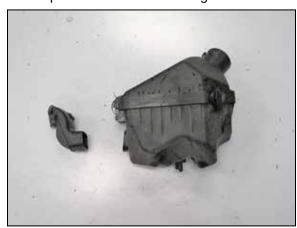
22. Remove the fresh air intake duct from the factory air filter housing.
