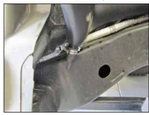
53. Install the duck bill fitting onto the port at the bottom of the corner tube and secure with the provided hose clamp.
