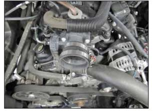
29. Install the provided coupler (084034) onto the throttle body and secure with the provided hose clamp.
