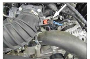
2. Release the red locking tap and then disconnect the inlet air temperature sensor electrical connection.
