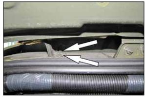
11. Lift up the cowl and then remove the two bolts that secure the fender to the inner cowl.
