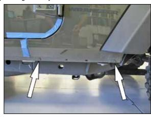
13. Remove the two lower fender bolts.
