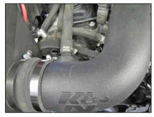
35. Connect the crank case vent hose as shown and secure with the provided hose clamp.
