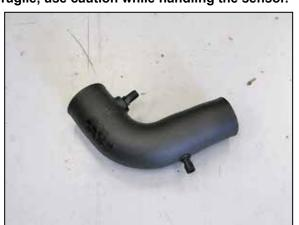
33. Remove the O-ring from the sensor and then install the sensor into the grommet installed into the  $K\&N^{\otimes}$  intake tube.
