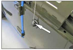
8. Remove the antenna mast.
