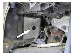
36. Remove the Insulation retaining nut shown.
