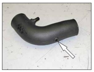
31. Install the provided grommet into the K&N® intake tube as shown.
