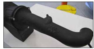
15. Install the K&N® intake tube assembly onto the K&N® airbox with provided hardware. Note the orientation of the K&N® intake tube.
