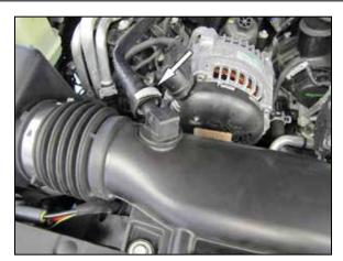
3. Disconnect the crank case vent line.
