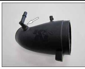
11. Install the provided 90° quick disconnect fitting into the K&N<sup>®</sup> intake tube as shown. **NOTE: Plastic NPT fittings are easy to cross thread. Install the vent fitting "hand" tight, then turn it two complete turns with a wrench.**
