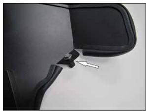
8. Install the nut insert onto the heat shield and secure with the provided hardware.
