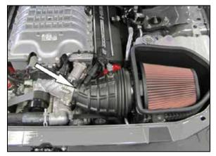
3. Loosen the hose clamp that secures the intake tube to the throttle body. NOTE: Some models will have a enclosed intake system, disassembly is the same for enclosed systems.
