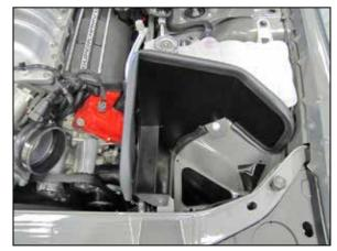
12. Install the provided coupling hose (KITHUMPHS12) onto the throttle body and secure with the provided hose clamp. Set the heat shield into position on the inner fender but do not secure at this time. **NOTE: Some models may have interference between the heat shield and A/C line. if this is the case the A/C line can be moved slight inward by applying pressure and slightly bending the aluminum line.**
