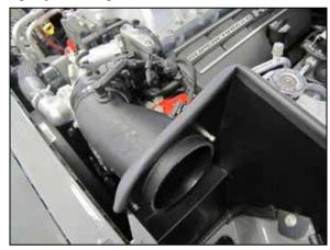
13. Install the K&N<sup>®</sup> intake tube into the coupling hose and heat shield and secure with the provided hardware to the heat shield.
