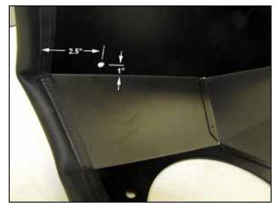
7a. On vehicles equipped with the CCV valve on the air filter housing lid, drill a 1/4"id hole 2.5" down from the top of the heat shield and 1.0" from the bend as shown. This hole will be used to secure the CCV valve to the heat shield.
