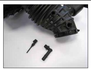
11. Remove the IAT sensor and quick connect CCV fitting from the factory intake tube. NOTE: Use caution while handling the inlet air temperature sensor as it is very fragile.
