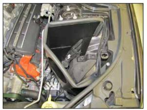
8. Install the heat shield so the mounting grommets engage with the factory mounting studs.
