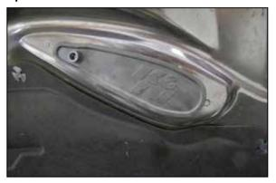
16. During wet conditions, install the provided hood vent block off to minimize water intrusion to the intake system. For Dodge vehicles, see step #17.
