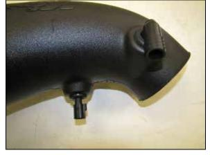
12a. On vehicles equipped with a CCV valve, install the provided 90deg union fitting into the K&N<sup>®</sup> intake tube as shown.
