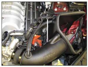
14c. Connect the factory CCV connector to the valve, route the 3/4" hose to the fitting installed into the intake tube as shown. Using the mounting tree tie wrap, secure the valve to the heat shield.
