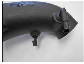
12. Remove the O-ring from the IAT sensor and then install the sensor into the K&N® intake tube as shown. Install the factory quick connect CCV fitting into the K&N<sup>®</sup> intake tube as shown.
