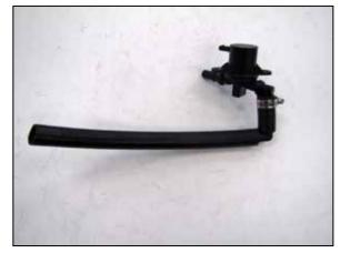
14b. remove the O-ring from the valve and then assemble the provided 3/4" hoses and 90deg. Union as shown. Secure the hose to the valve with the clamp provided.
