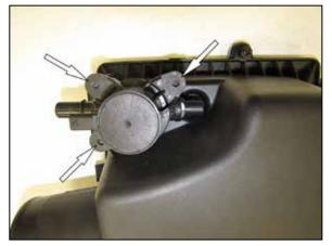
14a. On vehicles equipped with the CCV valve, carefully drill out the center of the plastic weld rivets that secure the valve and then remove the valve from the air filter lid.
