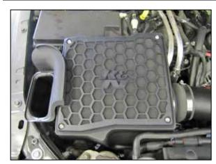
22. Install the filter lid onto the air filter housing and secure with the provided hardware.
