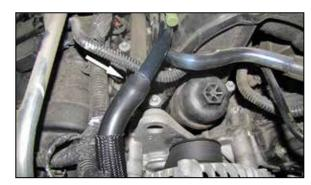
5. Disconnect the crank case vent flex line from the hardline at the connection shown.
