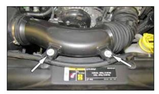
3. Remove the two bolts that secure the factory intake tube to the fan shroud.
