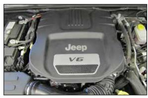
2. Lift up the engine cover to dislodge it from the mounting studs and then remove the cover from the engine.
