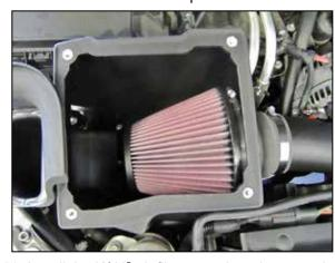
20. Install the K&N $^{\!0}$  air filter onto the adapter and secure with the provided hose clamp.
