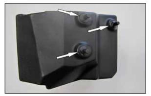
7. Install the three mounting studs provided onto the K&N® air filter housing using the provided hardware.
