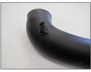
14. Remove the inlet air temperature sensor from the factory intake tube. Using the provided grommet install the inlet air temperature sensor into the K&N® intake tube.
