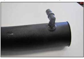
15. Install the provided 90° fitting into the K&N® intake tube as shown.
