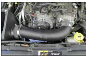
16. Install the provided hump coupler (08699) onto the K&N® intake tube and then install the assembly into the vehicle. Adjust the tube for best fit and then secure with the provided hose clamps. Reconnect the inlet air temperature sensor electrical connection.
