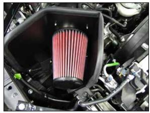
15. Install the air filter onto the intake tube and ire with the provided hose clari
