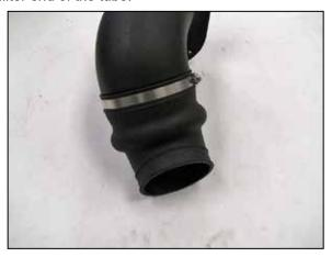
10. Install the flex coupler onto the intake tube and secure with the provided hose clamp. The coupler is keyed and can only be install in one location.
