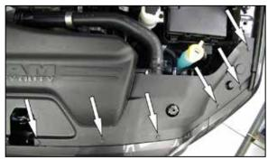
2. Remove the 14 push clips that secure the upper core support plastic cover and then remove the cover from the vehicle.
