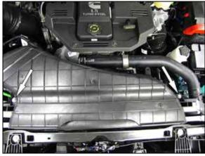
3. Remove the two bolts that secure the fresh air inlet duct to the core support and then remove the inlet from the vehicle.
