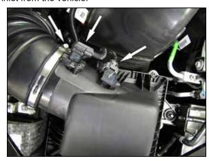
4. Loosen the hose clamp that secures the intake tube to the air filter housing and disconnect the electrical connections of the two air sensors.
