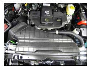
16. Install the K&N® fresh air duct into the heat shield and then install the factory portion of the fresh air duct and secure with the factory hardware.
