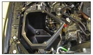
12. Install the K&N<sup>®</sup> filter housing into the vehicle so the mounting pins protrude through the grommets.
