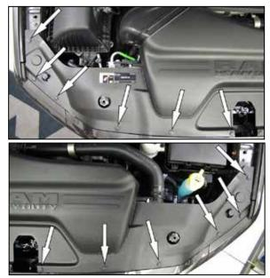
2. Remove the 14 push clips that secure the upper core support plastic cover and then remove the cover from the vehicle.
