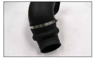
10. Install the flex coupler onto the intake tube and secure with the provided hose clamp. The coupler is keyed and can only be install in one location.
