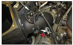
14. Reconnect the air sensor electrical connections.
