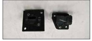
8. Remove the air sensors from the factory housing and install them into the K&N<sup>®</sup> sensor adapters using the provided hardware.
