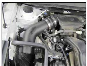
11. Install the K&N® intake tube through the heat shield and then secure it to the intake plenum using the coupler and hose clamps provided.
