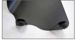
5. Remove the two factory mounting grommets from the factory air filter housing and install them into the K&N<sup>®</sup> heat shield as shown.
