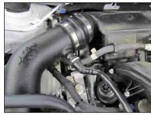
12. Connect the factory crank case vent hose to the quick connect fitting installed into the K&N® intake tube.
