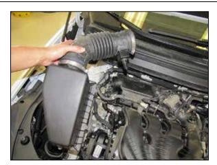
4. Loosen the hose clamp that secures the intake tube to the intake plenum. Disconnect the intake tube and then remove the complete intake system. NOTE: K&N Engineering, Inc., recommends that customers do not discard factory air intake.
