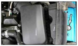
6. Remove the bolt that secures the factory air filter housing to the vehicle and then remove the housing from the vehicle.
