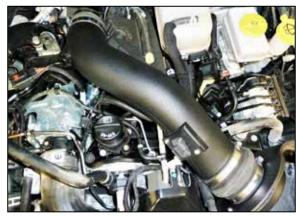
14. Install the K&N intake tube into the couplers, align for best fit and then secure the hose clamps.
