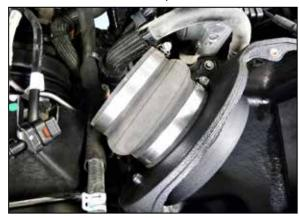
9. Install the provided hump coupler onto the filter adapter and secure with the provided hose clamps.
