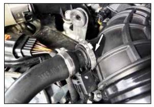
4. Release the one-time use clamp that secures the CCV hose to the factory intake hose and then desperate the CCV from the intake hose.
