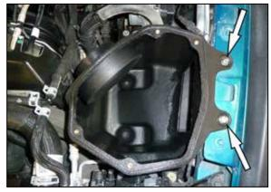
8. Set the K&N air filter housing assembly into the vehicle and secure with the provided hardware.
