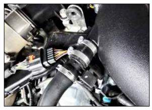
16. Using the provided hose and clamps, secure the CCV hose to the K&N intake tube.
