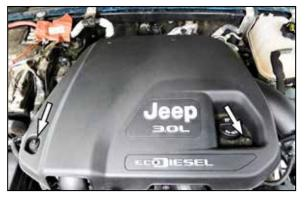
2. Remove the two bolts that secure the engine cover and then remove the engine cover from the vehicle.
