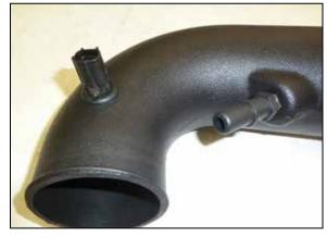
13. Install the provided CCV quick connect fitting into the K&N intake tube. Remove the IAT sensor from the factory intake tube, remove the O-ring from the sensor and then install it into the K&N intake tube using the provided grommet.
