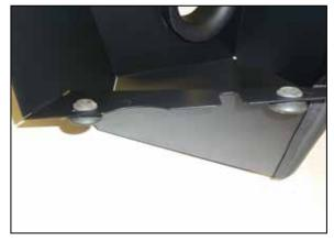
8. Remove two of the mounting grommets from the factory air filter housing and install them into the K&N heat shield as shown.
