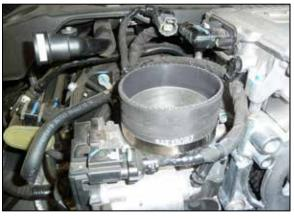
12. Install the provided straight coupler onto the throttle body and secure with the provided hose clamp.
