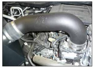
14. Install the K&N intake tube into the couplers, adjust for best fit and then secure with the provided hose clamps.
