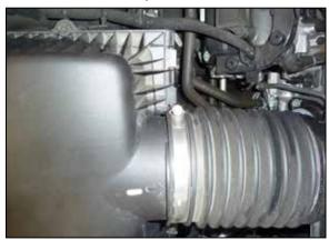
4. Loosen the hose clamp that secures the intake tube to the air filter housing. Remove the intake tube from the vehicle.
