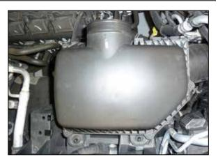
5. Pull the air filter housing up and remove it from the vehicle.
