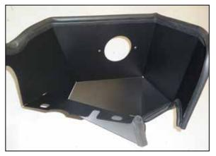
6. Install the edge trim onto the heat shield as shown. Some trimming of the edge trim will be necessary.
