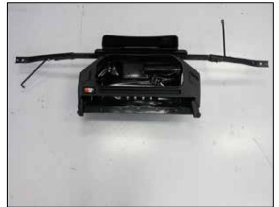
26. Secure the factory air filter housing support bracket to the K&N air filter housing using the provided hardware. Install the K&N logo into the filter housing.
