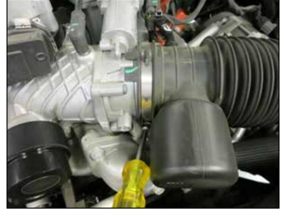
11. Loosen the hose clamp that secures the intake tube to the throttle body.
