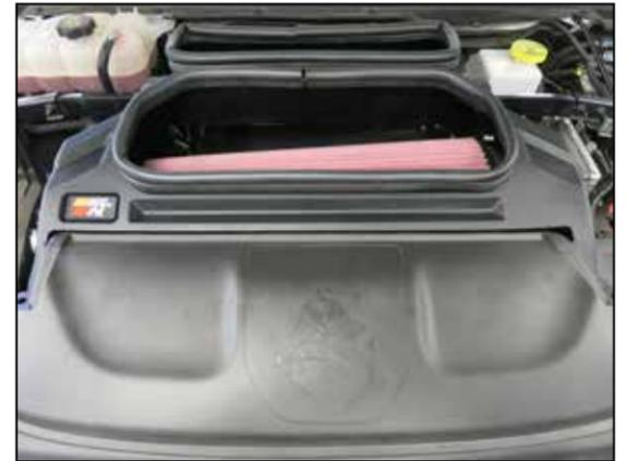
38. Reinstall the upper valence and secure with the factory retaining clips.
