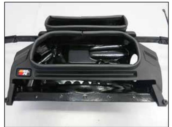
27. Install the provided edge trim onto the K&N air filter housing.
