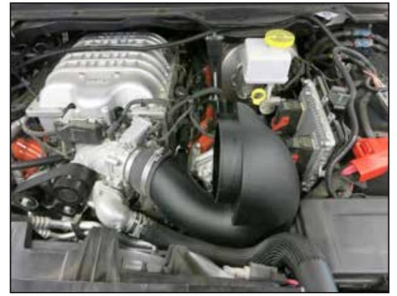
24. Install the K&N intake tube into the coupler at the throttle body but do not tighten the hose clamp to secure the tube.
