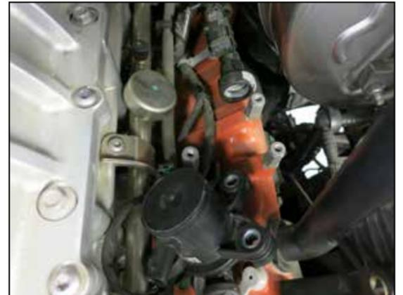
13. Disconnect the CCV line from the CCV switch at the quick connector.
