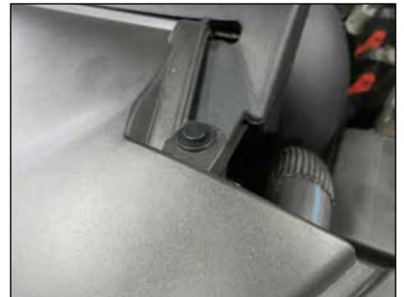
39. Install two provided retaining clips into the front into the front of the air filter housing through the valence.
