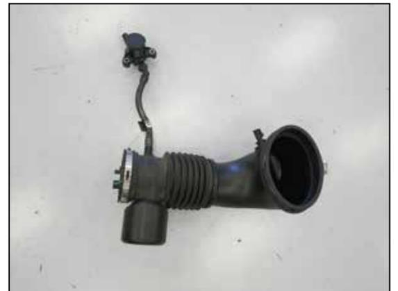
14. Remove the intake tube with the CCV switch and hose assembly from the vehicle.
