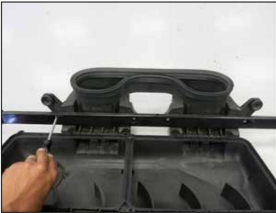
17. Remove the bolts that secure the air filter housing support bracket to the housing and set the support bracket aside.
