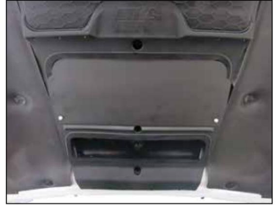
47. During severe inclement weather such as heavy rain or snow, K&N recommends install the provided forward fresh air block off plate using the provided hardware.
