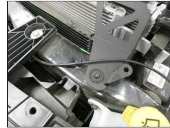
33. Secure the front air filter housing mounting bracket to the core support using the factory air filter housing mounting bolts.
