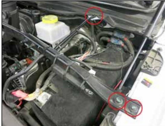
8. Remove the three bolts shown that secure the air filter housing mounting bracket to the driver side inner fender.
