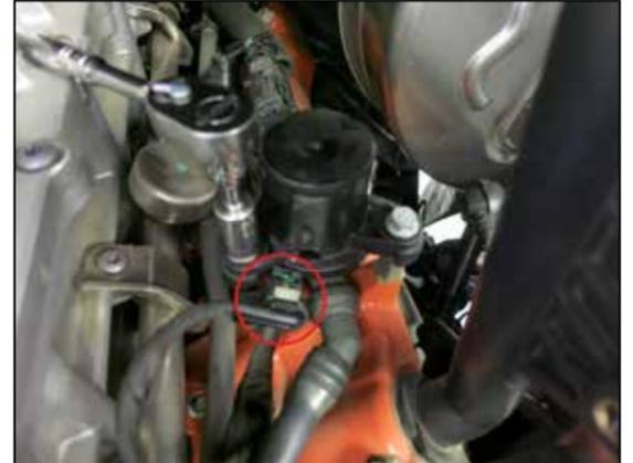
12. Disconnect the CCV switch electrical connection. Remove the mounting bolts that secure the CCV switch to the valve cover.
