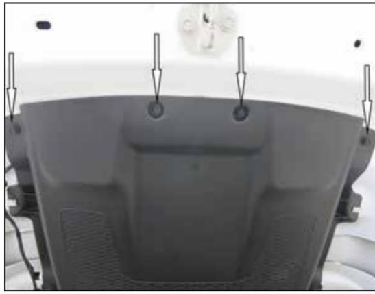
19. Remove the four bolts that secure the front of the factory fresh air intake duct.
