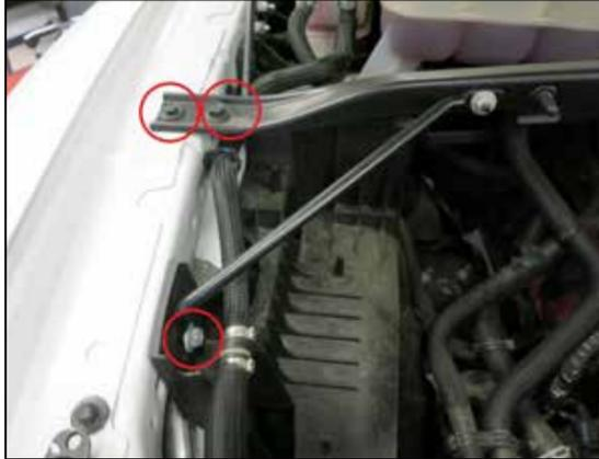
7. Remove the three bolts shown that secure the air filter housing mounting bracket to the passenger side inner fender.
