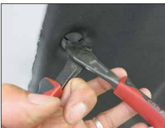
18. Cut the retaining clips that secure the left and right-side hood insulation panels. **NOTE: The clips will be destroyed during these process, new clips are provided to reinstall the insulation panels.**
