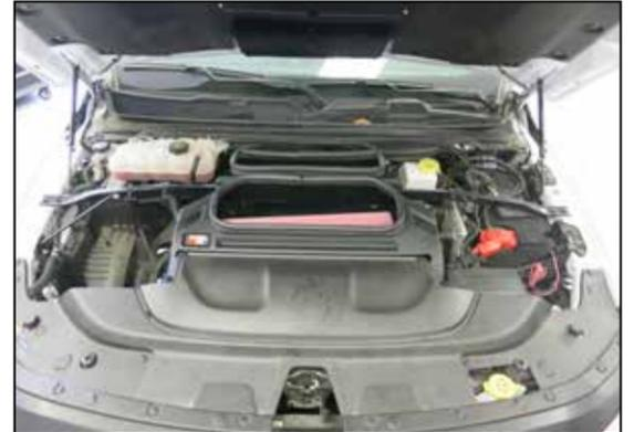
48. Reconnect the vehicle's negative battery cable. Double check to make sure everything is tight and properly positioned before starting the vehicle.
