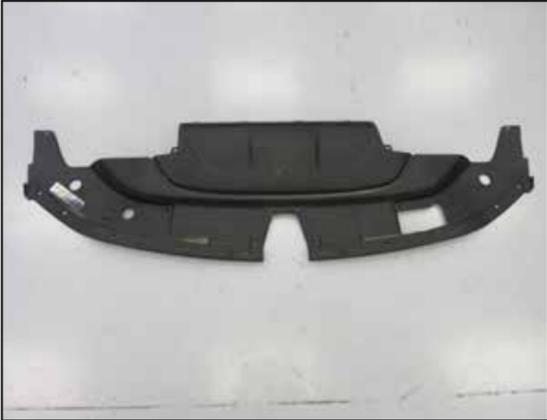
3. Remove the plastic fasteners from the upper valence and then remove the valence from the vehicle.
