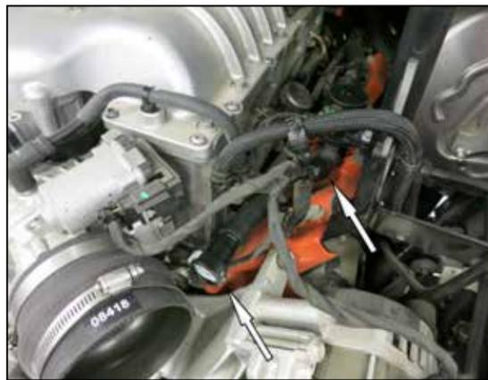
23. Assemble the provided CCV hose and quick connect fitting. Install the assembled CCV hose onto the CCV switch as shown.
