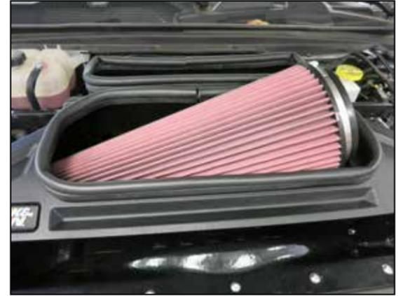
37. Install the K&N air filter into the housing and onto the intake tube, then secure with provided hose clamp.
