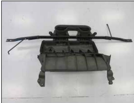
9. Remove the lower air filter housing and mounting bracket as an assembly.
