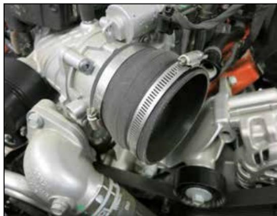
22. Install the provided coupler onto the throttle body and secure with the provided hose clamp.
