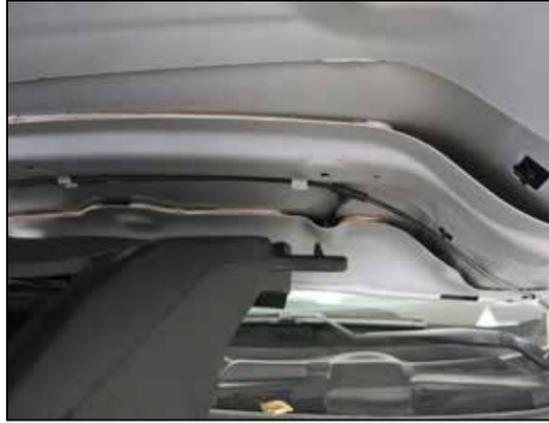
44. Rotate the fresh air duct up and align the mounting clips previously installed to the mounting holes in the hood.
