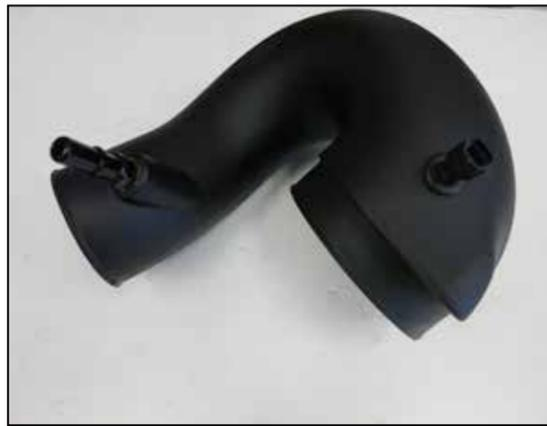
21. Remove the IAT sensor from the factory intake tube and install it into the K&N intake tube using the provided grommet. Install the provided quick connect fitting into the K&N intake tube as shown. **NOTES: The IAT sensor is fragile, use care when handling the sensor so as not to break it. The quick connect fitting npt tapered threads and will not tighten all the way down.**
