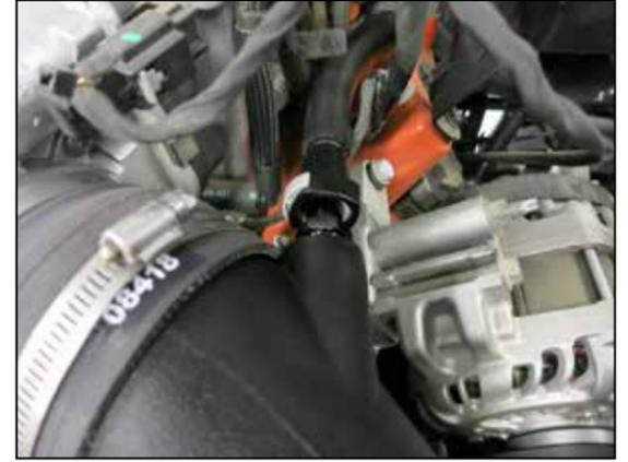
25. Connect the CCV quick connect fitting to the fitting installed into the K&N intake tube.
