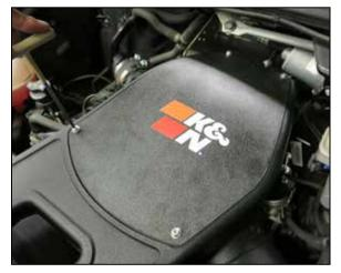
22. Install the K&N air filter housing lid and secure with the provided hardware.
