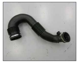
8. Loosen the clamp that secures the factory intake tube to the turbo and remove it from the vehicle.
