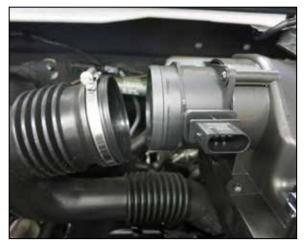
4. Loosen the hose clamp the secures the factory intake tube to the factory air filter housing and then disconnect the hose from the housing.
