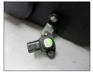
7. Disconnect the CCV sensor electrical connection.
