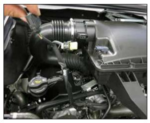
2. Disconnect the mass air sensor and sensor electrical connections and unhook the harness from the factory air filter housing.
