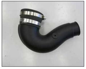
10. Install the provided step coupler onto the K&N intake tube and secure with the provided hose clamp. Install the provided grommet into the K&N intake tube.
