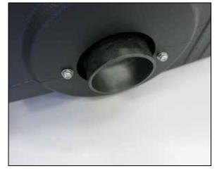
9. Install the provided radius filter adapter into the K&N air filter housing and secure with the provided hardware.
