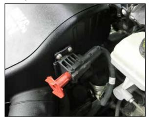
23. Attach the jump post positive terminal to the K&N filter housing using the provided hardware.
