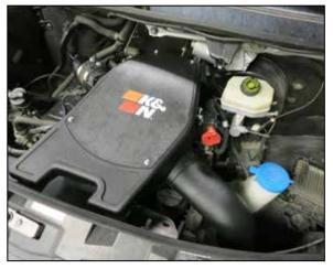
24. Reconnect the vehicle's negative battery cable. Double check to make sure everything is tight and properly positioned before starting the vehicle.
