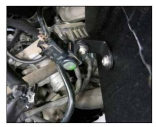
20. Reconnect the mass air sensor and sensor electrical connections.
