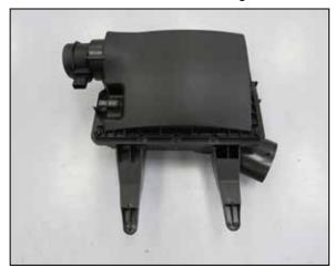
5. Lift the front of the air filter housing up to separate it from the mounting grommets, then while rotating the housing up and down to rotate it in the rear mounting grommets slide the housing towards the driver side until it is free of the rear mounts and remove it from the vehicle.
