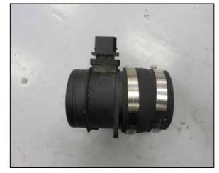
13. Install the provided step hose onto the inlet side of the mass air sensor and secure with the provided hose clamp. NOTE: Be sure the hose is on the inlet side of the sensor, If the sensor is installed the wrong direction the vehicle will not run properly, and the check engine light will be illuminated. There is an arrow embossed on the side of the housing showing the correct maf direction.
