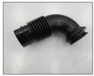
6. Pull up the Fresh air duct and remove it from the vehicle.
