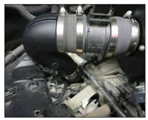
17. Install the K&N intake tube and mass air sensor assembly into the couplers, adjust for best fit and then secure with the provided hose clamps. **NOTE: Be sure the mass air sensor is installed in the correct direction. Is the sensor is installed backwards the vehicle will not run correctly and will illuminate the check engine light.**
