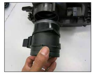
12. Remove the mass air sensor from the factory air filter housing.
