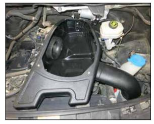
16. Install the K&N air filter housing into the factory housing mounts and guide the fresh air tube into the duct.
