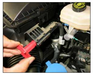
3. Disconnect the jump start positive post from the air filter housing and set aside.
