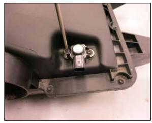
14. Remove the sensor from the factory air filter housing lid.
