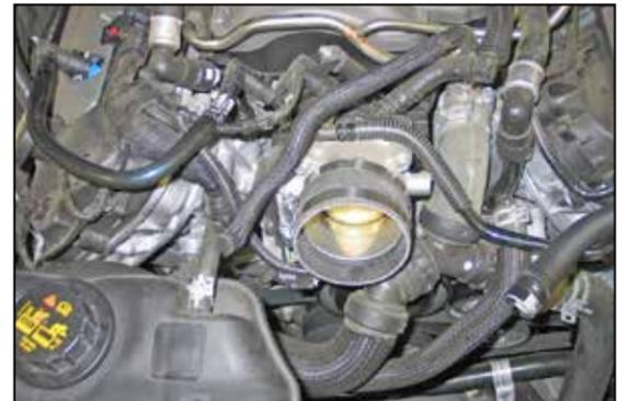
19. Install the provided silicone hose (08698) onto the throttle body and secure with the provided hose clamp.
