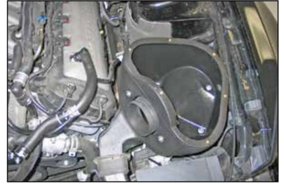
17. Set the K&N® airbox into the vehicle so that the mounting studs slide into the mounting holes, and then secure with the hardware provided.
