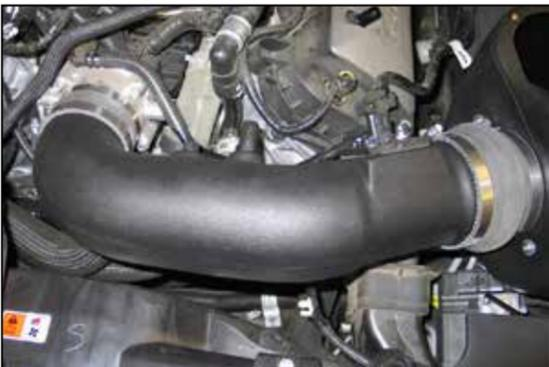
26. Install the K&N® intake tube into the silicone hose at the airbox and then into the silicone hose at the throttle body; secure with the provided hose clamps.
