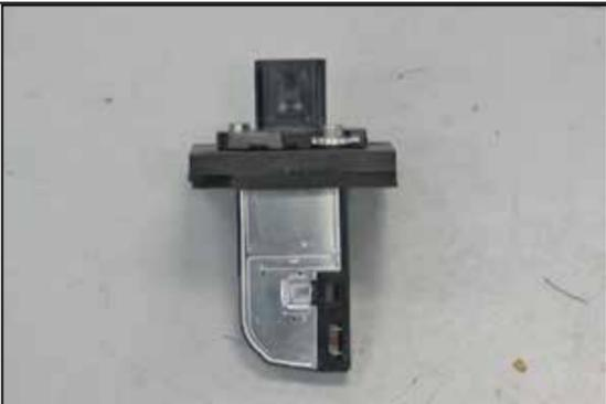
24. Install the mass air sensor into the K&N® adapter and secure with the provided hardware.
