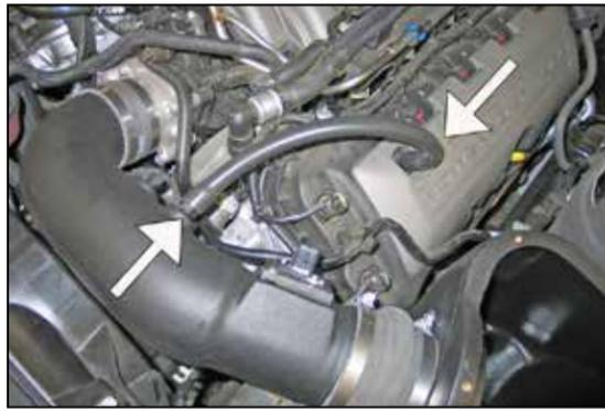
27. Install the crankcase vent hose to the fitting on the K&N® intake tube and onto the valve cover. Vehicles equipped with an EVAP vent line, connect it to the fitting installed in the K&N® intake tube.
