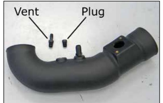
21. On vehicles that have an EVAP vent line attached to the intake tube, install the 3/8" vent fitting into the K&N® intake tube. On vehicles that do not have the EVAP vent line attached to the intake tube, install the NPT plug into the intake tube.
