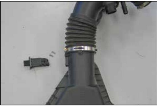
22. Remove the two bolts securing the mass air sensor into the factory intake tube and then remove the mass air sensor from the intake tube.
