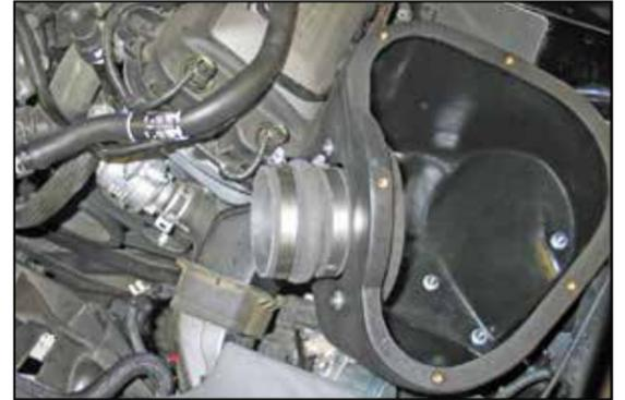
18. Install the provided silicone hose (08418) onto the filter adapter and secure with the provided hose clamp.
