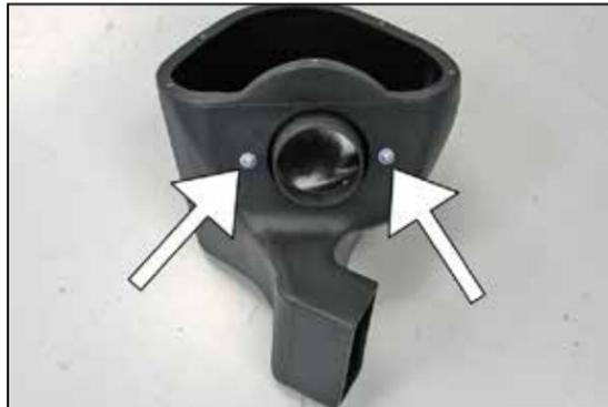
14. Install the filter adapter into the airbox and secure with the provided hardware.
