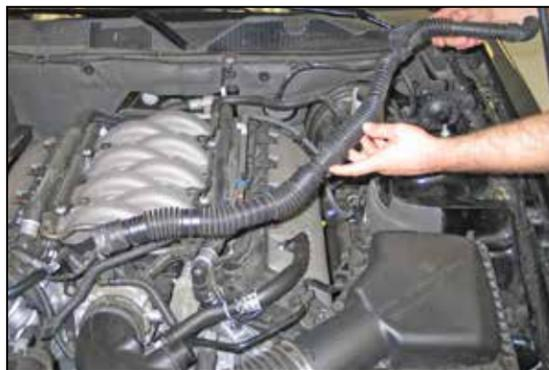
4. Release the clamp which secures engine pulse hose to the intake tube then remove the engine pulse hose from the vehicle.
