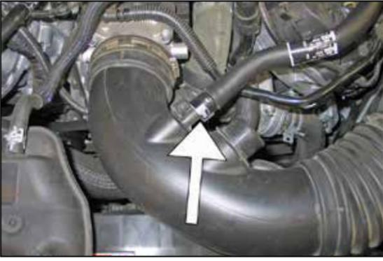
7. Disconnect the crankcase vent hose from the factory intake tube and valve cover port and remove the vent tube from the vehicle.
