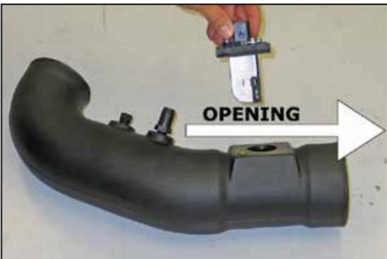
25. Install the mass air sensor assembly into intake tube and secure with the provided hardware.
