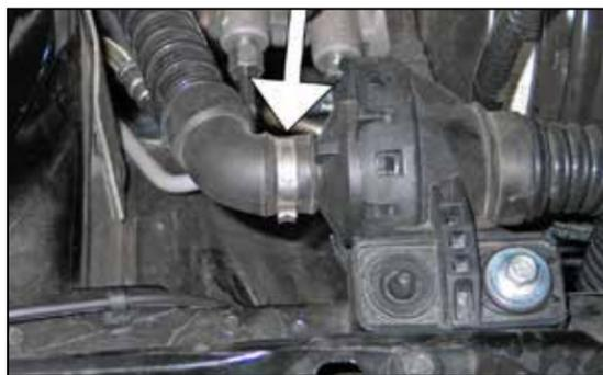
3. Cut the clamp that secures the engine pulse hose to the drum and disconnect the hose from the drum.
