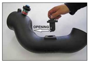
12. Using the provided grommet, install the factory filter minder into the K&N<sup>®</sup> intake tube. Then install the mass air sensor assembly into the K&N<sup>®</sup> intake tube as shown.
