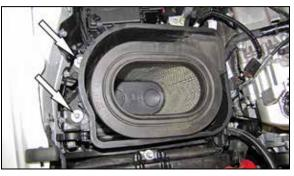
4. Remove the two bolts that secure the lower air filter housing to the mounting bracket and remove the lower filter housing.
