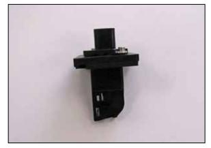
11.Install the mass air sensor into the K&N<sup>®</sup> adapter and secure with the provided hardware.
