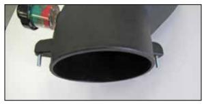
13. Install the two provided mounting studs into the  $K\&N^{\otimes}$  intake tube as shown.
