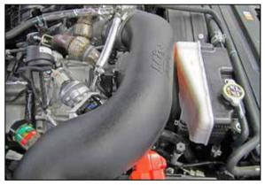
18. Reconnect the mass air sensor electrical connection and use the provided tie wrap to secure the wiring harness.
