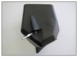
6. Using the provided hardware, secure the mounting stud to the K&N<sup>®</sup> air filter housing as shown.
