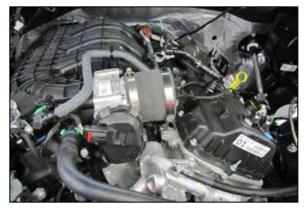
6. Install the provided coupling hose (084055) onto the throttle body and secure with the provided hose clamp.
