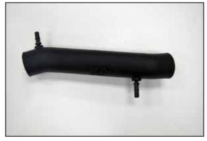
8. Install the provided quick connect fittings into the  $K\&N^{\mbox{\tiny $\$$}}$  intake tube as shown.
