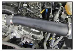
11. Connect the factory vent lines to the quick connect fittings installed into the K&N<sup>®</sup> intake tube.
