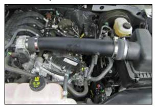
9. Install the K&N<sup>®</sup> intake tube into the Coupler at the throttle body and then onto the coupler at the air filter housing. Secure the upper air filter housing and then adjust the tube for best fit and secure with the provided hose clamps.
