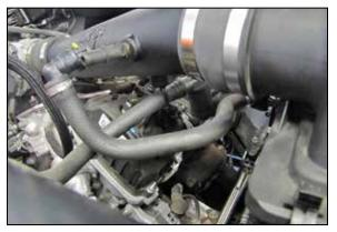
10. Secure the vent hose to the K&N<sup>®</sup> intake tube with the provided mounting head tie wrap.
