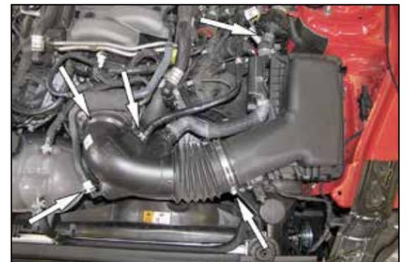
5. Release the retaining clip securing the EVAP vent lines and then disconnect the lines from the intake tube. Locate the hose clamp that secures the Sound tube to the Sound drum located on the driver side strut tower. Release the clamp by cutting with pliers and then disconnect the sound tube from the drum. Loosen the hose clamps that secure the intake tube to the throttle body and air filter housing and then remove the tube from the vehicle.
