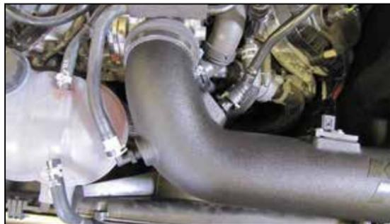
16. Connect the EVAP and crank case vent lines to the fittings installed into the K&N® intake tube.
