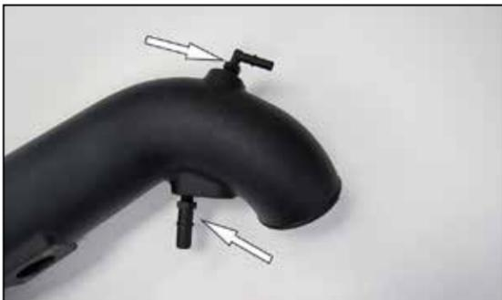
9. Install the provided fittings into the K&N® intake tube as shown. **NOTE: Plastic NPT fittings are easy to cross thread. Install the vent fitting "hand" tight, then turn it two complete turns with a wrench.**
