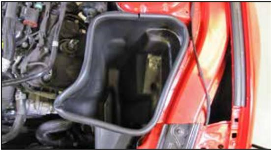
8. Install the provided edge trim onto the K&N® air filter housing. Install the K&N® air filter housing into the vehicle and secure with the provided hardware. **NOTE: Some trimming of the edge trim will be necessary.**
