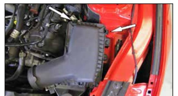
6. Release the clips that secure the upper air filter housing and then remove the upper air filter housing from the vehicle.
