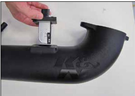
12. Install the mass air sensor assembly into the K&N® intake tube as shown and secure with the provided hardware. **NOTE: Be sure to install the maf sensor in the correct direction as shown in the photo. The vehicle will not run properly if the sensor is installed backwards.**
