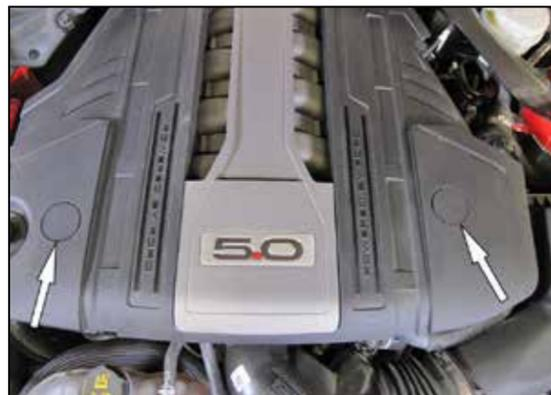
3. Remove the fastener covers on the engine cover, remove the two nuts that secure the cover and then remove the cover from the engine.
