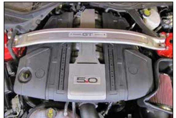
20. Reinstall the engine cover and secure with the factory hardware, reinstall the nut covers. Reinstall the strut tower brace and secure with the factory nuts.
