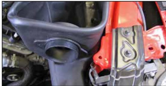
14. Install the filter adapter into the K&N® air filter housing and then install the tube gasket onto the adapter.
