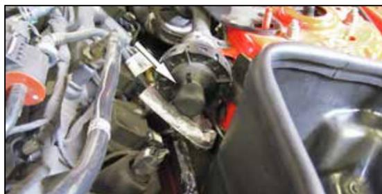
17. Install the provided cap onto the sound drum as shown.
