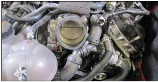
13. Install the provided coupling hose (08699) onto the throttle body and secure with the provided hose clamp.
