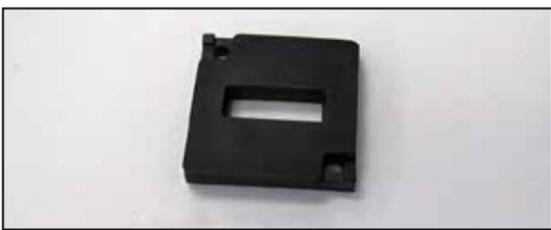
10. Install the provided gasket onto the K&N® mass air sensor adapter.
