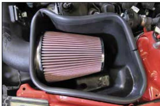
18. Install the K&N® air filter onto the filter adapter and secure with the provided hose clamp. **NOTE: Drycharger® air filter wrap; part # RF-1020DK is available to purchase separately. To learn more about Drycharger® filter wraps or look up color availability please visit <http://www.knfilters.com>®.**
