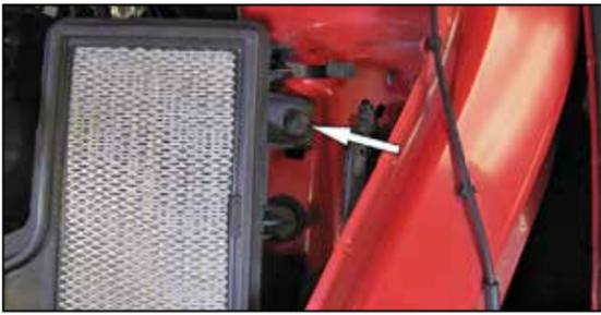
7. Remove the bolt that secures the air filter housing to the inner fender and then remove the lower air filter housing from the vehicle.
