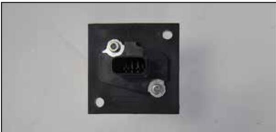
11. Remove the mass air sensor from the factory air filter housing and install it into the K&N® adapter using the provided hardware.
