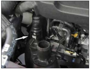
4. Release the locking ring and then disconnect the crank case vent tube from the intake tube.
