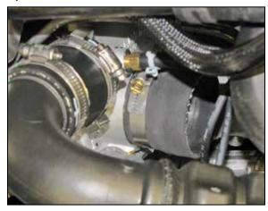
15. Install the provided hose (08638) onto the turbo and secure with the provided hose clamp.
