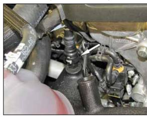
21. Connect the crank case vent hose to the fitting installed into the K&N® intake tube.
