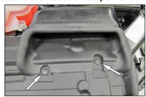
6. Remove the two clips that secure the fresh air intake duct to the core support.
