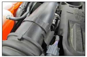
3. Disconnect the mass air wiring harness clip from the intake tube.
