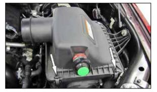
5. Release the two clips that retain the factory upper air filter housing and the remove the upper housing from the vehicle.
