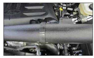
20. Secure the mass air sensor wiring harness to the K&N® intake tube.
