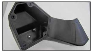
10. Secure the K&N® fresh air intake duct to the lower air filter housing using the hardware provided
