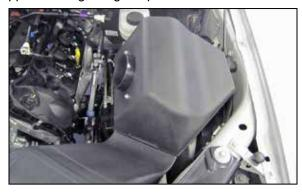
14. Install the upper filter housing assembly onto the previously installed lower housing so the mounting studs insert into the grommets.
