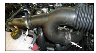
5. Loosen the hose clamps that secure the intake tube to the turbo inlet pipes and then remove the intake tube from the vehicle.
