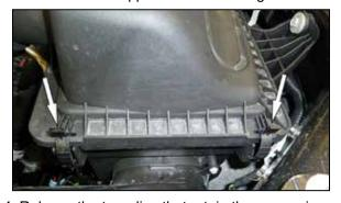
4. Release the two clips that retain the upper air filter housing and then remove the upper housing from the vehicle.
