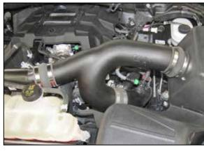
19. Install the K&N® intake tube into the couplers, align for best fit and then secure with the provided hose clamps.
