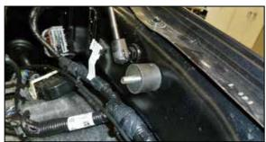
11. Install the provided rubber mounted stud into the factory filter housing mounting location as
