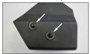
8. Install the provided mounting studs onto the K&N® lower filter housing using the provided hardware.
