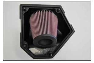
15. Install the air filter assembly into the upper air filter housing and secure with the provided hardware.
