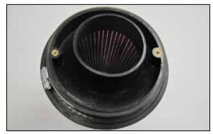
14. Install the filter adapter into the filter and secure with the provided hose clamp.
