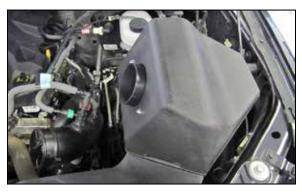
16. Install the upper filter housing onto the lower housing so the mounting studs insert into the mounting grommets.
