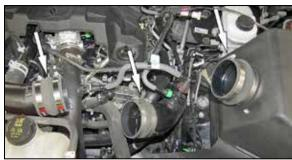
17. Install the hump coupler (08699) onto the filter adapter, hump coupler (087121) onto the upper (passenger side) turbo inlet pipe and coupler (07861) onto the lower (Drivers side) turbo inlet pipe and secure with the provided hose clamps.
