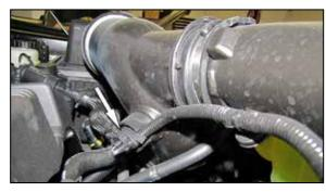
2. Disconnect the inlet air temperature sensor electrical connection.
