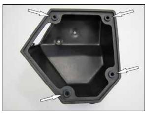
9. Install the four mounting grommets provided into the K&N® lower air filter housing as shown.
