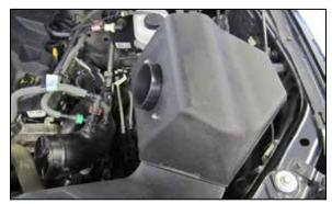
15. Install the K&N® lid/filter assembly onto the lower filter housing so the mounting studs engage into the mounting grommets
