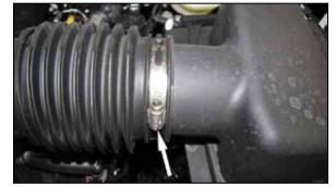
3. Loosen the hose clamp that secures the factory intake tube to the factory upper air filter housing.
