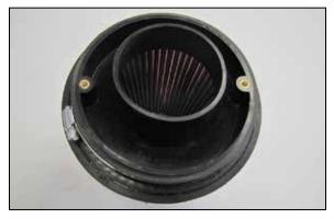
13. Install the filter adapter into the filter and secure with the provided hose clamp.
