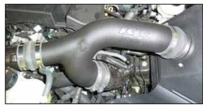
19. Install the K&N® intake tube into the couplers for the turbo inlet pipes and the filter adapter, adjust the tube for best fit and then secure with the provided hose clamps.
