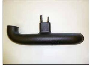
21. Install the provided vent fittings into the K&N® intake tube as shown.
