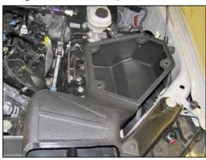
14. Install the K&N® air filter housing assembly into the vehicle and secure to the rubber mounted stud using the provided hardware.
