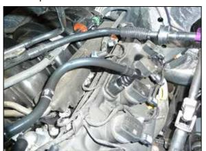
23. On vehicles that the CCV hose connects to the valve cover in front of the first coil pack, use the factory CCV hose and connect it to the fitting installed into the K&N® intake tube.
