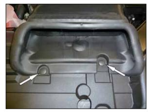
7. Remove the two clips that secure the fresh air intake duct to the core support.
