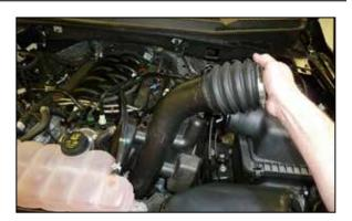
5. Remove the factory intake tube from the vehicle.
