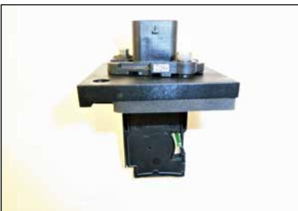
10. Install the gasket onto mass air sensor adapter and then remove the mass air sensor from the factory filter housing and install it into the K&N adapter using the provided hardware.
