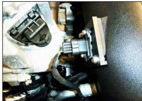
17. Reconnect the mass air sensor electrical connection.
