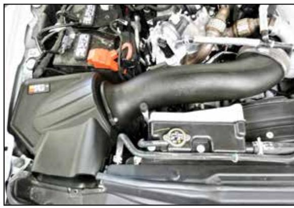
15. Install the intake assembly onto the lower air filter housing and guide the pins of the lid into the grommets installed into the lower housing. Once the pins are aligned with the grommets push the lid down to engage.
