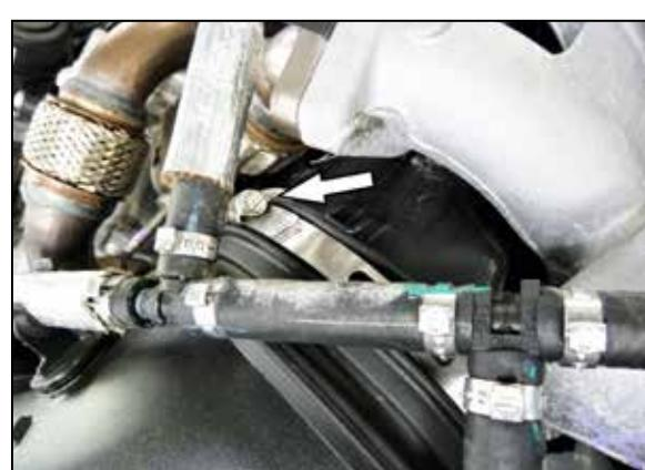
3. Loosen the hose clamp that secures the factory intake tube to the turbo inlet pipe.
