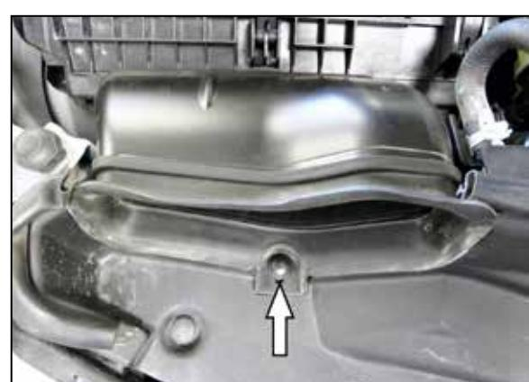
5. Remove the pin that secures the fresh air intake duct and then remove the duct from the vehicle.
