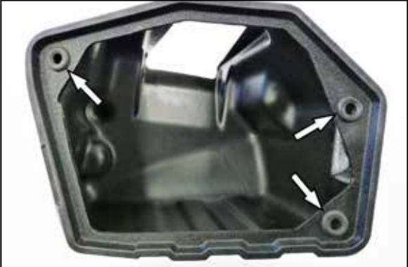
8. Install the three provided grommets into the K&N filter housing as shown.
