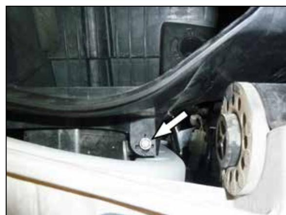
6. Remove the bolt securing the air filter housing and then remove the housing from the vehicle.
