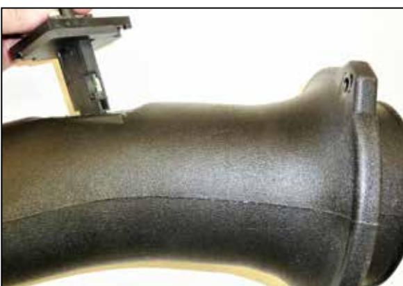
11. Install the mass sensor assembly into the K&N intake tube, be sure to install the sensor in the correct position so the opening of the sensor is pointed towards the filter end of the intake tube.
