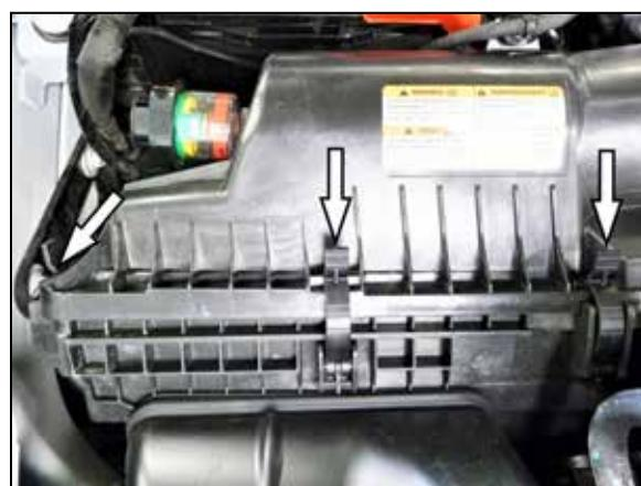
4. Release the three clips that secure the air filter housing lid and then remove the lid, intake tube and air filter from the vehicle.
