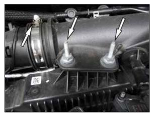
9. Loosen the hose clamp that secures the factory intake tube to the turbo inlet. Remove the hardware that secures the factory intake tube to the engine. This hardware will be reused with the K&N intake system.
