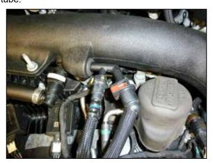
24. Connect the ejector line fittings to the ejector and secure the factory retaining locks.
