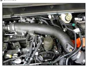
20. Install the K&N intake tube into the couplers at the filter adapter and turbo inlet, adjust the tube for best fit and secure with the provided hose clamp and factory hardware.
