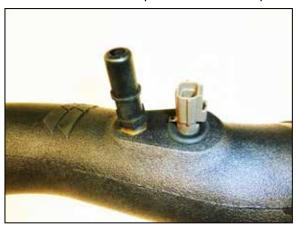
18. Remove the IAT sensor from the factory air filter housing, remove the O-ring from the sensor and then install the sensor into the K&N intake tube using the provided grommet. Install the provided CCV fitting into the K&N intake tube. **NOTE: The IAT sensor is fragile, use caution while handling the sensor.**
