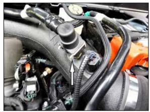
25. Reinstall the factory vent, secure the safety lock and reconnect the electrical connection.
