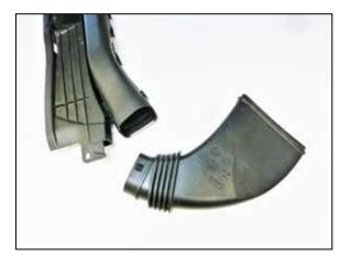
3. Separate the two sections of the fresh air intake duct, set the section that connects to the factory air box aside as it will not be used with the K&N intake system.
