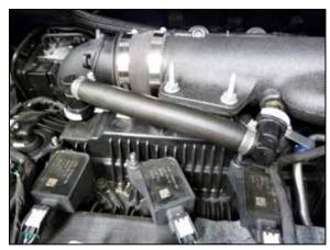
23. Install the CCV assembly onto the valve cover port and the fitting installed into the K&N intake tube.
