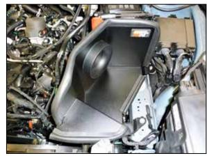
15. Install the heat shield into the vehicle so the mounting posts insert into the factory air filter housing mounting grommets.
