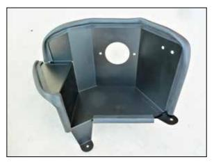
12. Install the edge trim onto the heat shield as shown. NOTE: the edge trim will be cut into three sections of 32", 12" and 6".
