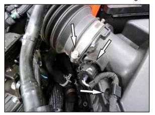
5. Loosen the hose clamp that secures the factory intake tube to the air filter housing. Disconnect the IAT sensor electrical connection and unhook the wiring harness from the air filter housing.
