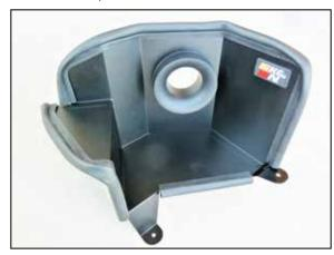
13. Using the provided hardware secure the filter adapter into the heat shield as shown. Install the K&N badge into the holes of the heat shield.
