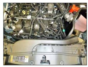
27. Reinstall the factory fresh air duct and secure with the factory pushpins.
