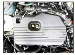
4. Remove the hardware that secures the engine cover and then remove the cover from the engine.
