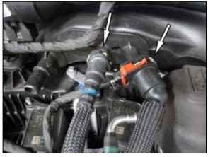
8. Release the red and yellow safety lock clips on the ejector vent lines and then release the clips that secure the ejector lines and disconnect them from the intake tube.
