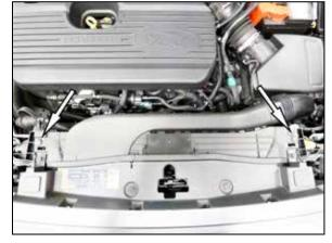
2. Remove the two pushpins that secure the fresh air intake duct and then remove the duct from the vehicle.
