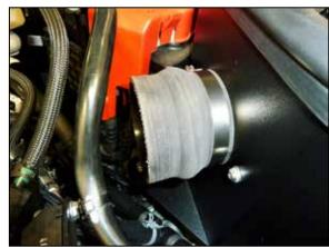
16. Install the provided hump hose onto the filter adapter and secure with the provided hose clamp.
