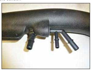
19. Install the remaining CCV fitting into the K&N intake tube as shown. Install the provided ejector fitting into the K&N intake tube using the provided grommet.
