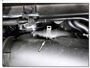
10. Release the spring clamp that secures the BOV hose to the factory intake tube and disconnect the BOV hose from the intake tube. Remove the complete stock intake tube from the vehicle.
