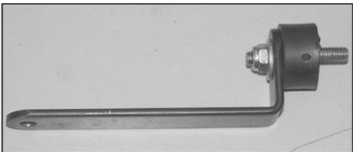
14. Install the rubber-mounted stud onto the heat shield mounting bracket (07091) and secure with the provided hardware as shown.
