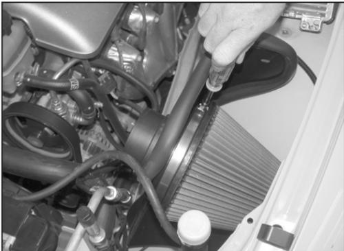
13. Install the heat shield assembly onto the inner fender and start the mount bolts in the air box mounting pin holes, then place the K&N® air filter into position. Tighten the heat shield mounting bolts, then install the K&N® air filter onto the filter adapter and secure with the provided hose clamp.
