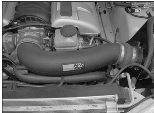
18. Install the K&N® intake tube into the silicone hose attached to the throttle body and then onto the mass air sensor. Secure with the provided hose clamps as shown.
