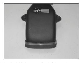
14. Install the supplied silicone hose (08619) onto the K&N Intake Tube and secure with the supplied hose clamp.
