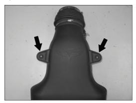
12. Remove the two mounting grommets shown from the stock intake tube.
