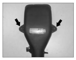
13. Install the mounting grommets removed in step #11 into the K&N Intake Tube mounting holes.
