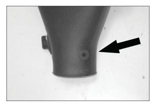
10. Install the provided grommet into the K&N Intake Tube as shown.
