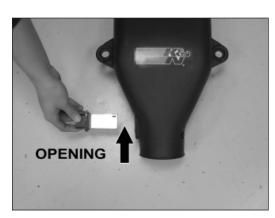
7. Install the mass air sensor into the K&N Intake Tube as shown.
