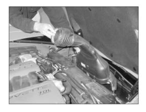
5. Pull the intake tube off of the throttle body and dislodge the intake tube from the mounting pins on the radiator cover. Then remove the complete intake assembly from the vehicle.
