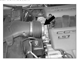
4. Loosen the hose clamp that secures the intake tube to the engine throttle body.
