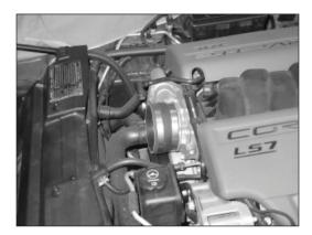
16. Install the silicone hose (08761) onto the throttle body and secure with the provided hose clamp.
