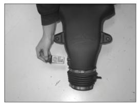
6. Remove the two screws which secure the mass air sensor in the stock intake tube and then remove the sensor as shown.
