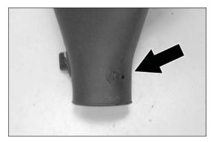
11. Install the crank case vent fitting removed in step #9 into the grommet installed into the K&N Intake Tube during step #9 as shown.
