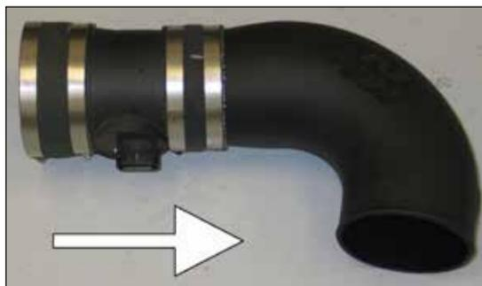
19. Install the mass air sensor assembly onto the K&N intake tube as shown.
