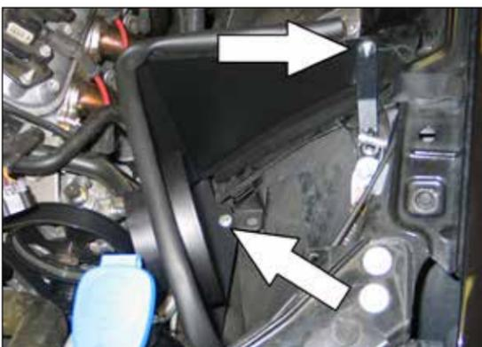
13. Install the heat shield assembly into the vehicle and secure it to the mounting bracket installed in step #10 and to the air box mounting stud location.
