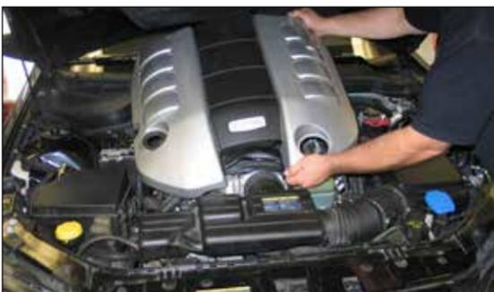
2. Remove the oil fill cap and then remove the engine cover from the engine as shown. Reinstall the oil fill cap.
