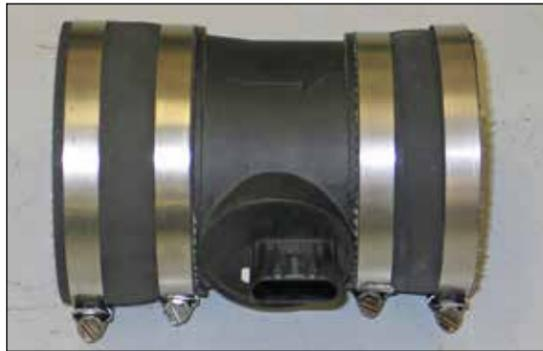
17. Install the provided silicone hose (08536) onto the mass air sensor and secure with the provided hose clamp.
