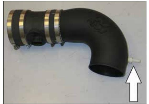
20. Install the crankcase fitting into the K&N intake tube as shown.
