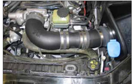
21. Install the K&N intake tube with mass air sensor into the silicone hose at the throttle body and onto the intake tube on the filter adapter. Rotate and adjust the intake tubes for proper fit and then secure the assembly with the hose clamps.
