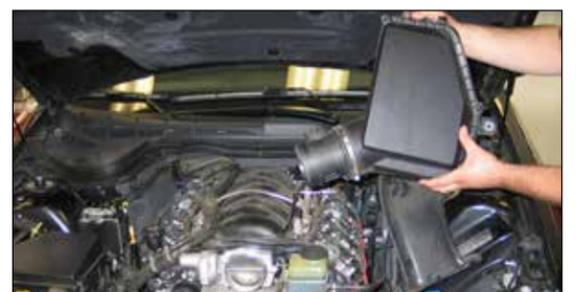
8. Remove the complete air box assembly from the vehicle.
