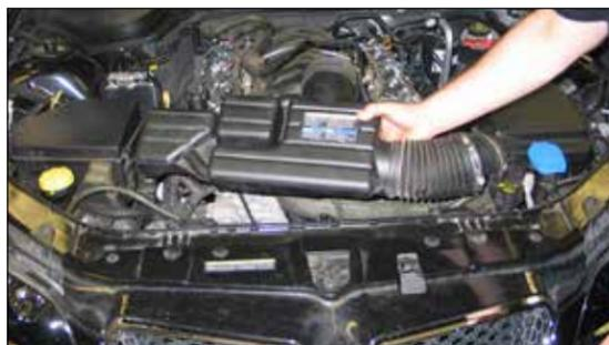
5. Remove the complete stock intake tube assembly from the vehicle as shown.
