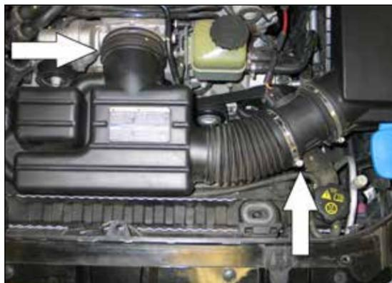
4. Loosen the two hose clamps which secure the stock intake tube to the throttle body and mass air sensor.
