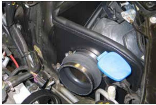
15. Install the provided silicone hose (08418) onto the filter adapter and secure with the provided hose clamp.
