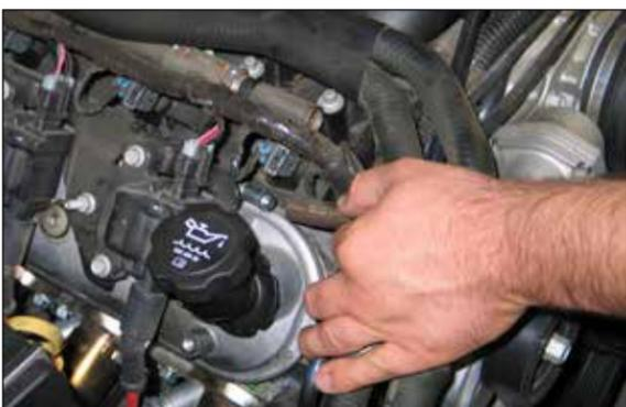
3. Disconnect the crank case vent hose from the valve cover as shown.
