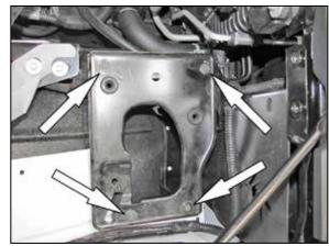
7. Remove the four bolts securing the air box mounting tray and then remove the tray from the
