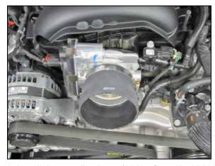
13. Install the coupling hose (08497 for 5.3L, 08418 for 6.2L) onto the throttle body and secure with the provided hose clamp.
