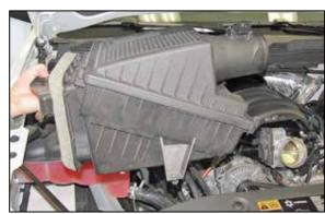
6. Pull up the air box to release it from the mounting grommets and then remove the factory air box from the vehicle.
