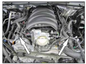
12. Remove the two factory crank case vent tubes from the vehicle.
