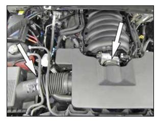
4. Loosen the two hose clamps securing the intake plenum to the factory air box and to the throttle
