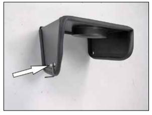
12. Install the heat shield mounting bracket (070712A) onto the heat shield using the provided hardware and spacer.
