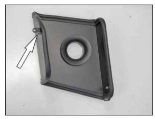
13. Install the heat shield mounting bracket (07805A) onto the heat shield using the provided hardware and spacer.
