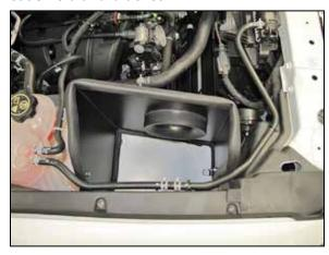
14. Install the heat shield into position and secure with the two of the factory nuts removed in earlier steps.
