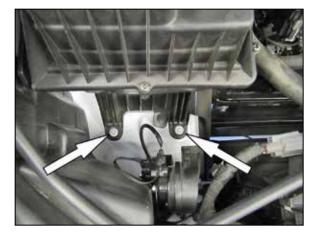
7. Remove the two bolts securing the air filter housing to the inner fender.
